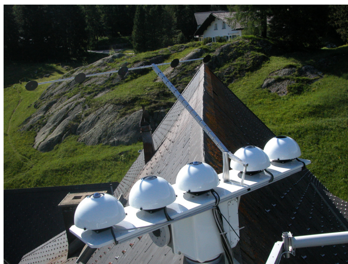
Figure 1 World infrared standard group of Pyrgeometers (WISG) at PMOD/WRC
