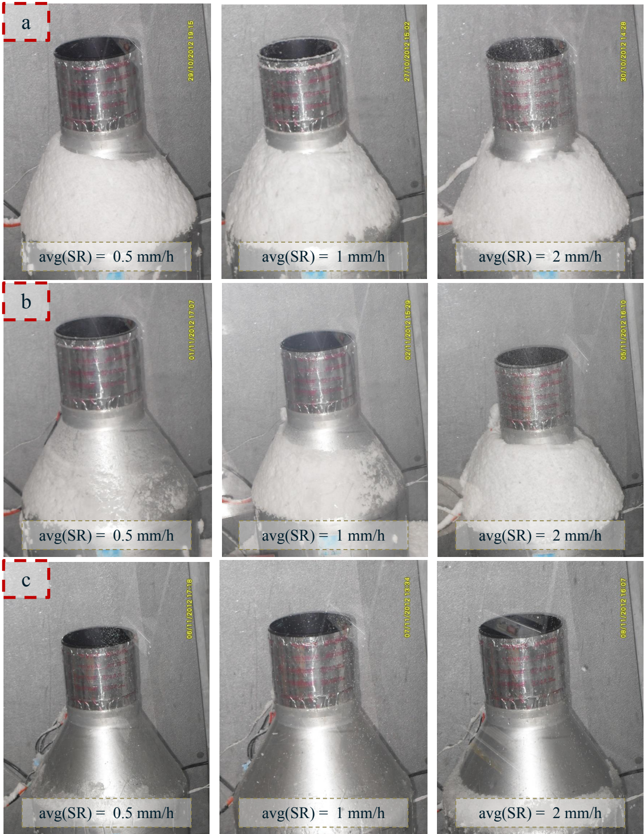
Fig. 5: Snow accumulation of the GEONOR T200B case after 1 mm of equivalent water. The gauge was equipped with an internal and an external AC heater stripe (2000W) managed by the modified CRN algorithm for three different environmental temperatures: a) \text{avg}(T_{\text{air}}) = -10^{\circ}\text{C} ; b) \text{avg}(T_{\text{air}}) = -5^{\circ}\text{C} ; c) \text{avg}(T_{\text{air}}) = -2^{\circ}\text{C}
