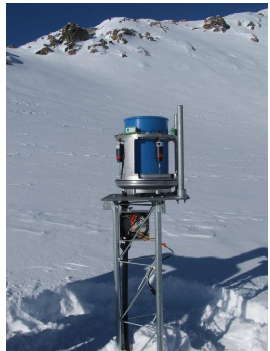
Photo 10: Weighing Gauge 2 - cover removed
