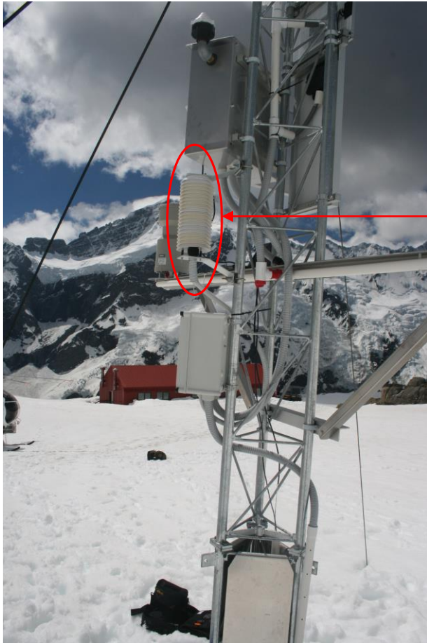
Photo 16: Air temperature and relative humidity sensor location on mast
