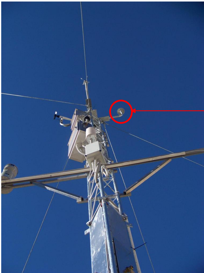
Photo 17: Solar radiation sensor location viewed from the base of the mast
