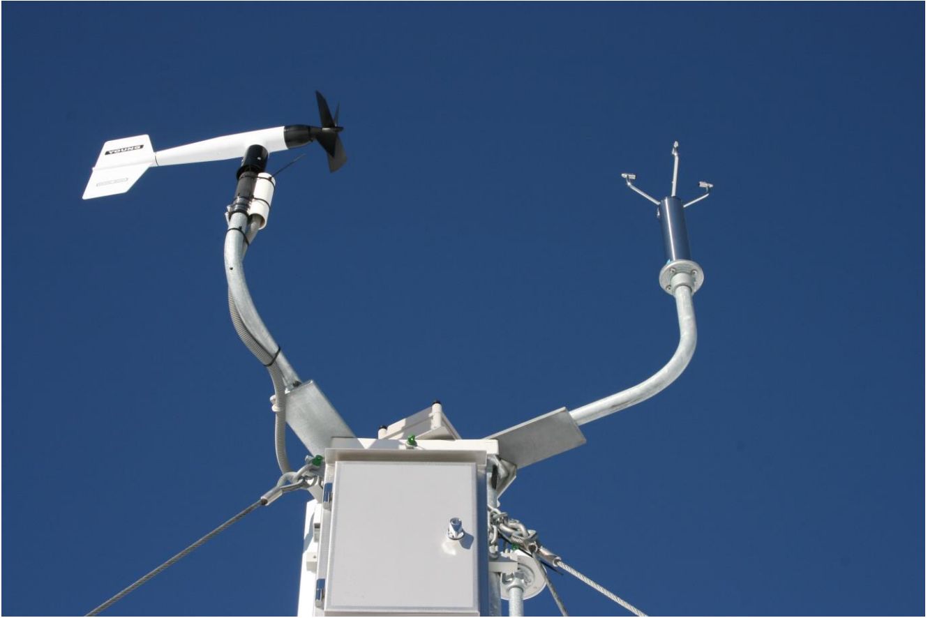
Photo 15: RM Young Wind Monitor. Vaisala ultra-sonic wind sensor (right hand instrument in this picture) no longer used
