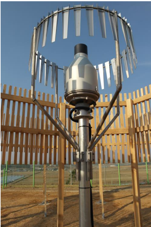
Photo of installation - Geonor gauge with Single-alter shield inside DFIR (North)
