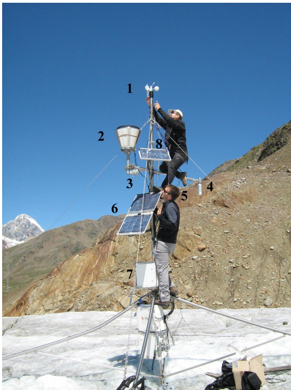
FIGURE 6: AWS1 Forni photographed from the South (summer time) during one of the periodic maintenance activities. The instruments are marked with numbers: (1) wind speed and direction, (2) rain gauge, (3) net radiometer CNR1, (4) sonic ranger, (5) thermo-hygrometer, (6) solar panels, and (7) barometer inside the data-logger box. From summer 2009 the AWS is online through a radio link and a GSM modem. The communication system is supported by a dedicated solar panel (8) and a gel battery 30 Ah.
