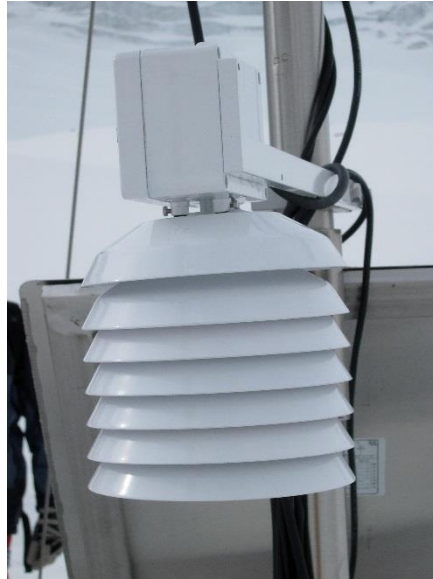
FIGURE 24: Detailed picture of the thermo-hygrometer.
