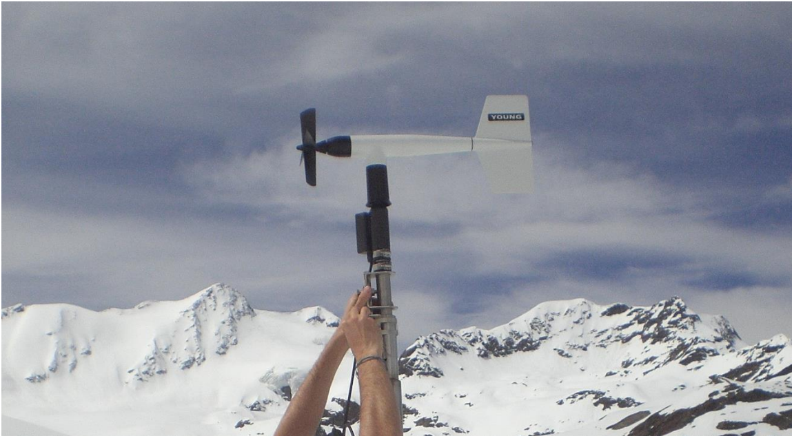
FIGURE 36: Detailed picture of the anemometer.
