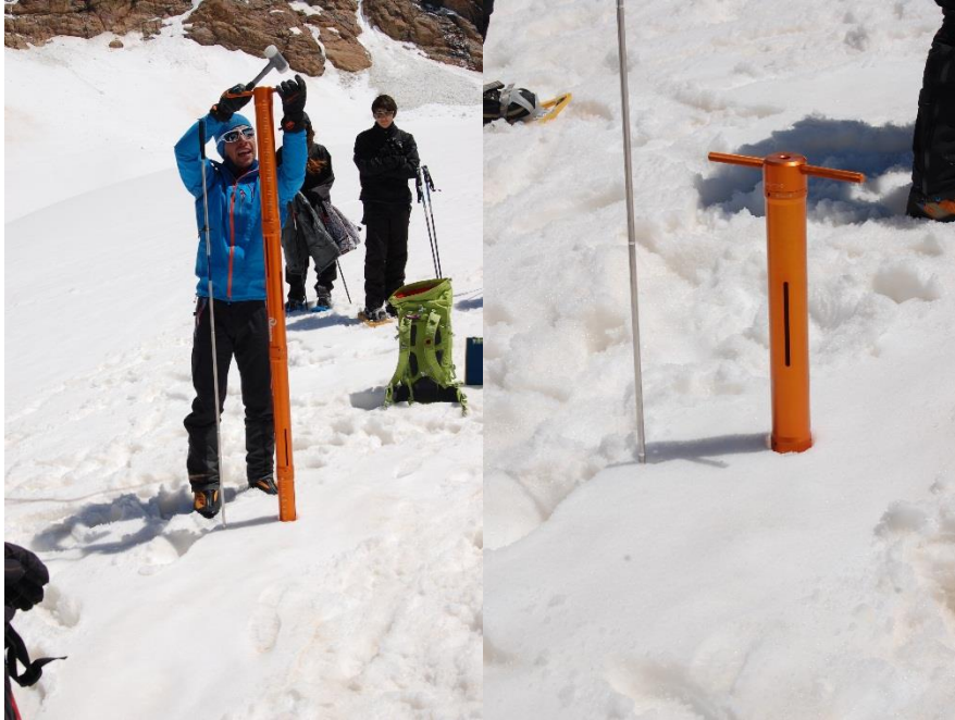
FIGURE 16: Detailed picture of the Enel-Valtecne snow weighing tube during measurements performed near to the AWS Forni SPICE.
