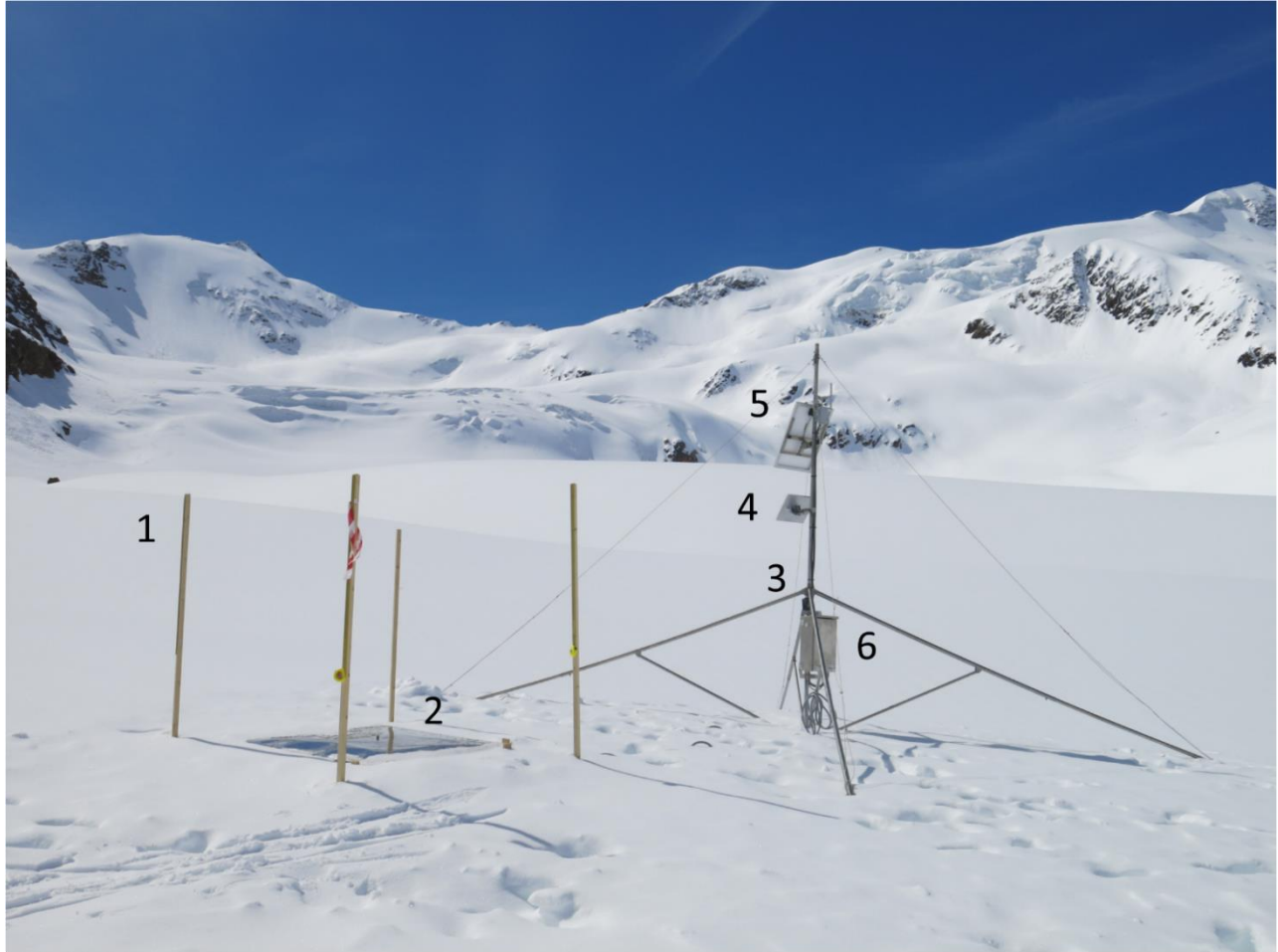
FIGURE 9: AWS Forni SPICE photographed from the North-East (after the installation on 6 th May 2014). The instruments are marked with numbers: (1) graduated stakes, (2) snow pillow, (3) automated camera, (4) antenna for the telecommunications, (5) solar panel, and (6) the data logger box.
