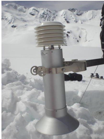
FIGURE 19: Detailed picture of the Sommer sonic ranger installed at the AWS1 Forni on 6 th May 2014.
