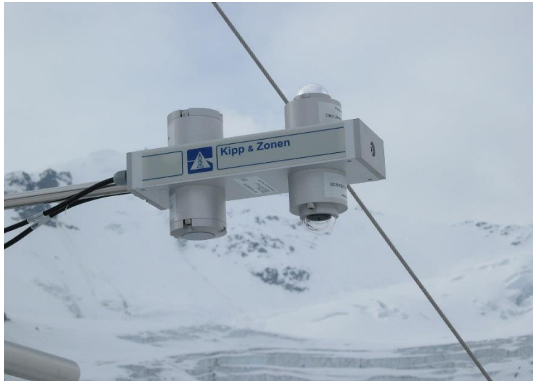
FIGURE 29: Detailed picture of the net radiometer.
