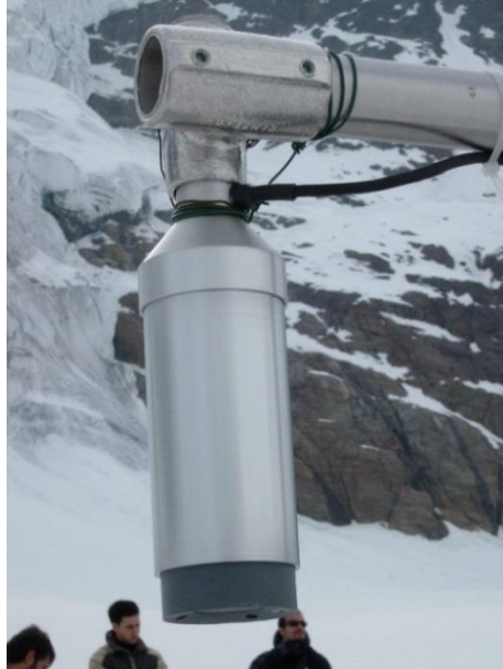
FIGURE 17: Detailed picture of the Campbell sonic ranger installed at the AWS1 Forni in autumn 2005.
