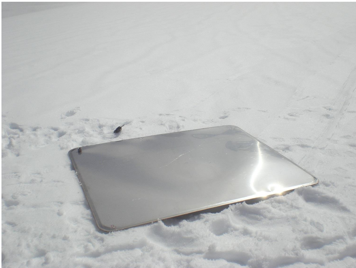
FIGURE 22: Detailed picture of the snow pillow downfacing side.
