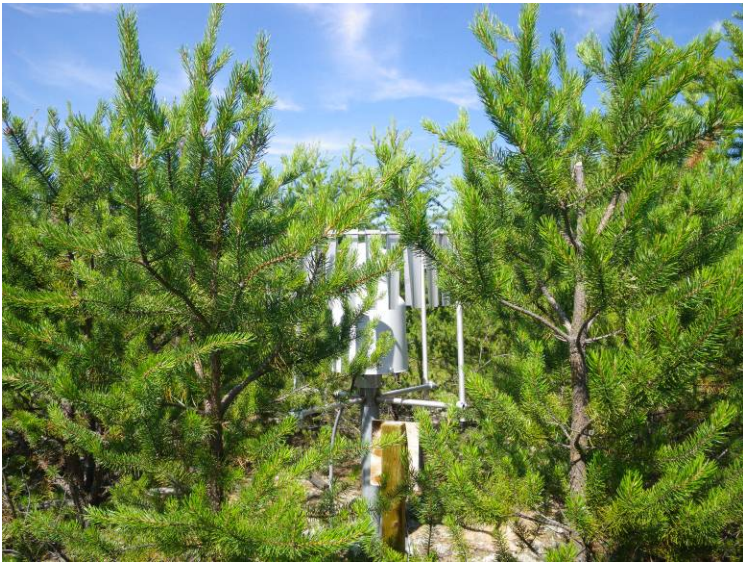
Bush shielded gauges. Pluvio2 (left) and Geonor T-200B (right)
