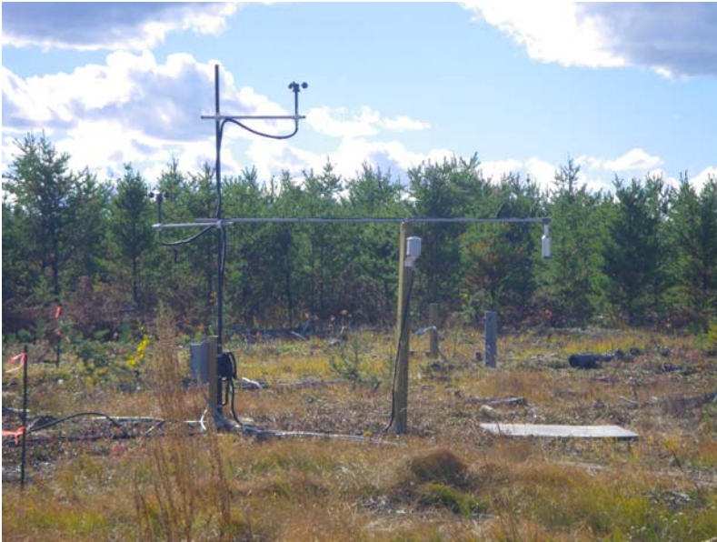
Unspirated HMP45C Temp/RH sensor (white radiation shield in centre) at C8
