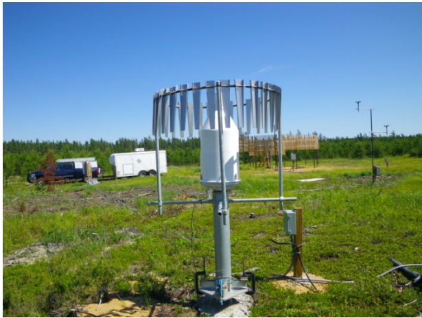
Geonor T-200B3M 1500mm gauge on C5 looking west (top left), north (top right), east (bottom left) and south (bottom right)
