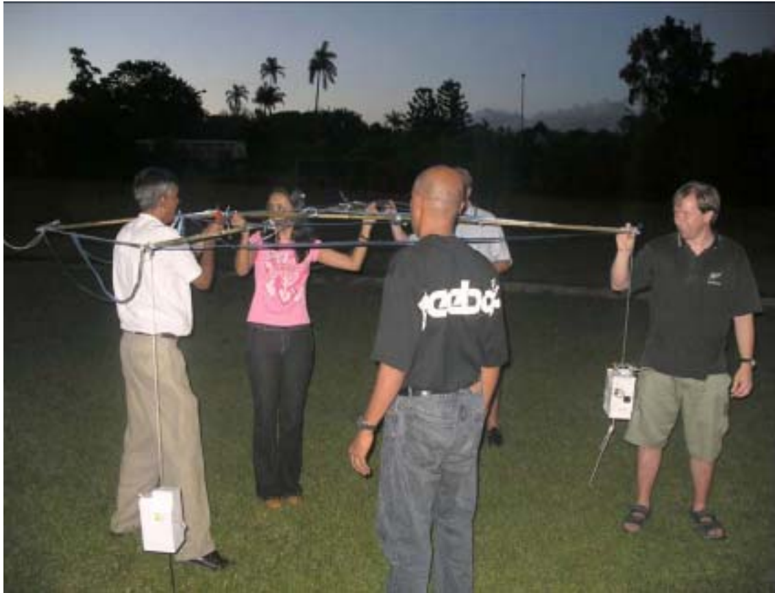
Fig. 3.1 Graw and Sippican 3-thermistor radiosondes ready for a nighttime intercomparison of the Vaisala-Sippican-Graw radiosonde group on the bamboo cross support rig.
