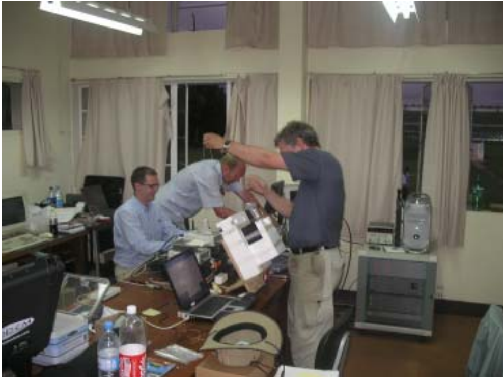
Fig. 3.2(a) Preparing Vaisala RS92 and Snow white for a night time flight. The PCs on the left hand bench are STAR (Mauritius) operational monitor, Laser ceilometer, and GPS water vapour data loggers. On the central bench Modem ground system + pre-flight check box, + Vaisala ground system + pre-flight check near the window, Meteorolabor radiosonde preparation + ground system behind this, and near the window the data logger and radar electronics for the cloud radar.
