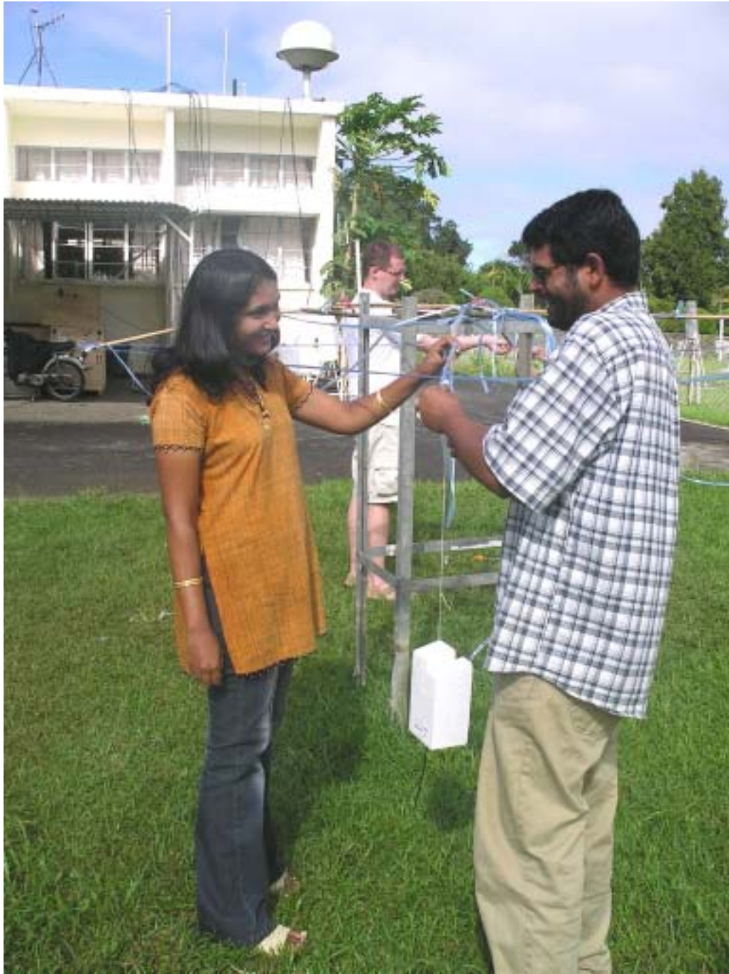
Attaching Graw radiosonde to flight rig
