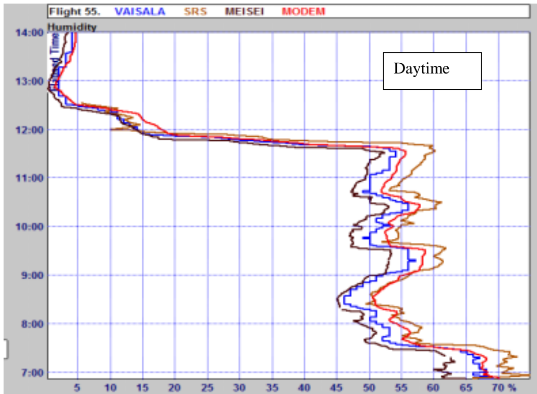
Fig. 10.3(a) Sample of detailed vertical structure from an individual flight, Meisei-Modem-Vaisala group plus Snow White, centered at about 3.5 km above the ground.
