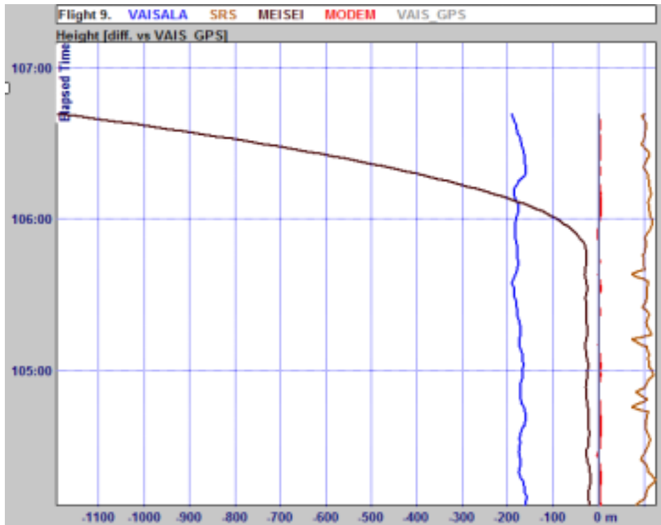
Fig. 7.2 Typical Meisei geopotential height error in the minute preceding balloon burst. These errors were hidden when using the WSTAT processing package
