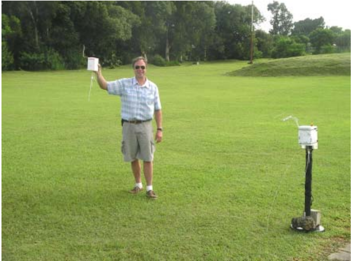
LMS-5 radiosonde + Sippican Multi-thermistor on stand.
