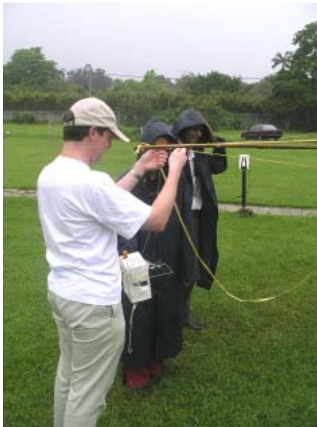
Multi-thermistor radiosonde in wet pre-launch conditions. The thermistors were shielded from the rain until immediately before launch.
