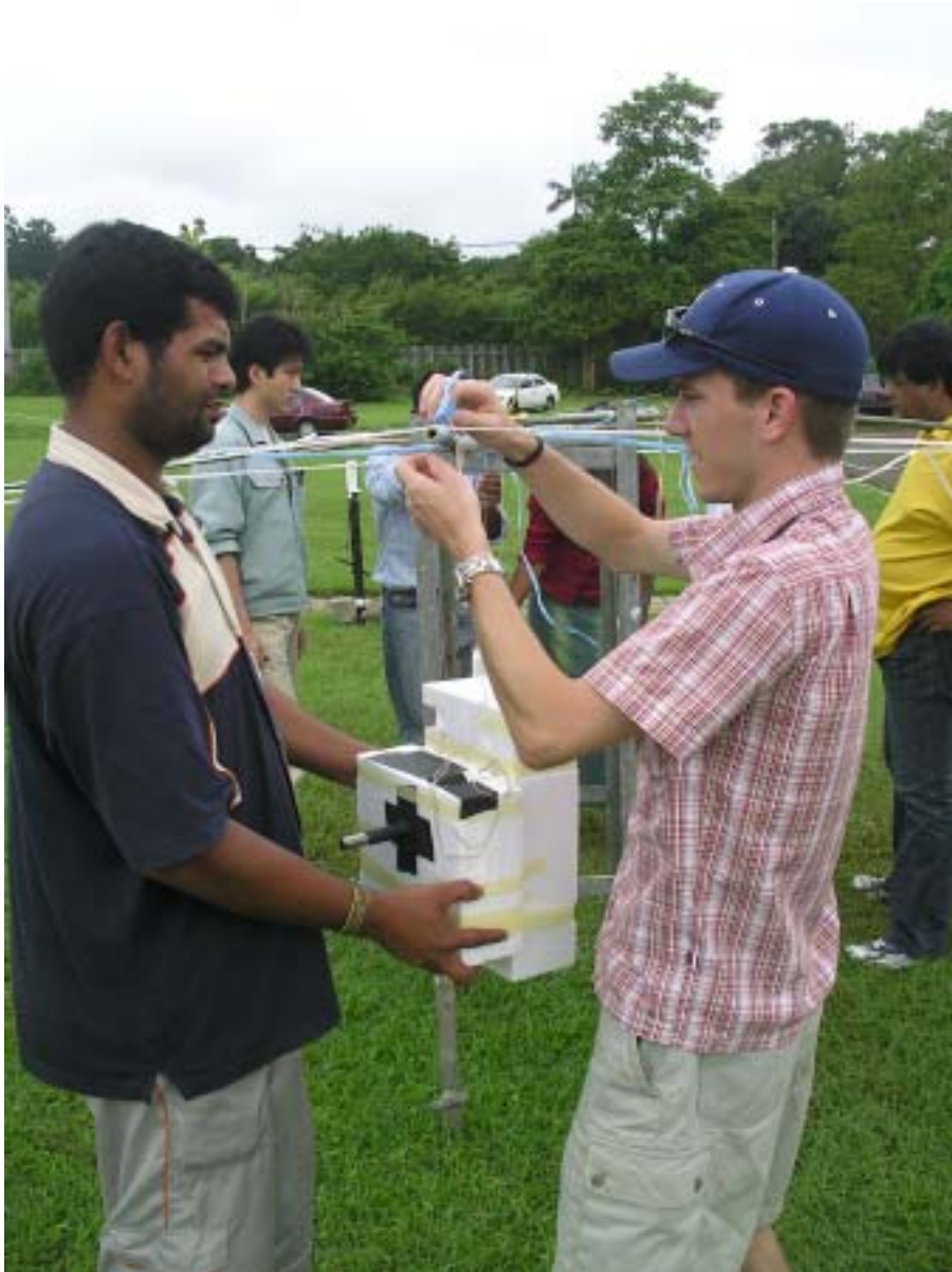
“Daytime” SRS + Snow White, with entrance to internal duct through side pipe in order to alleviate rain /cloud contamination of the duct.
