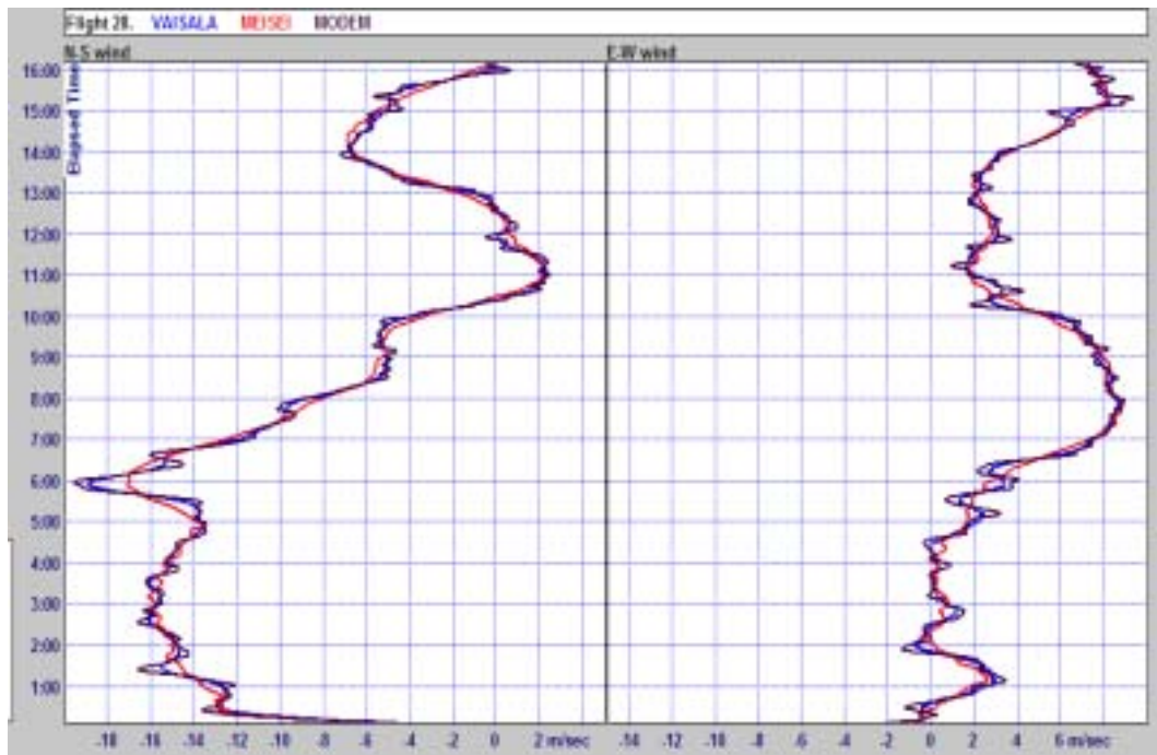
Fig. 6.1(a) Example of comparison between N-S and E-W wind components from Flight 28, showing the difference in filtering between MODEM, Vaisala and Meisei winds. Meisei winds were smoothed to the greatest extent and MODEM winds smoothed the least.
