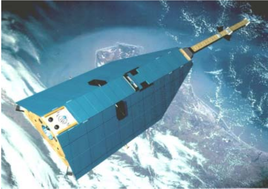
Fig. 12.6 CHAMP satellite which measures - among other geophysical parameters - the occultation parameters of GPS satellites.
