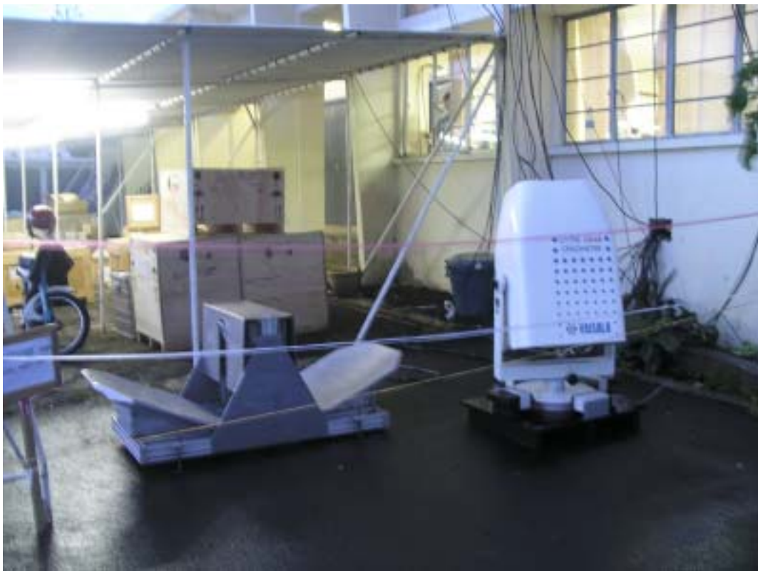
Fig. 12.1(a) Vaisala CT75K lidar ceilometer plus Rutherford Appleton Laboratory 78 GHz fmcw cloud radar (centre of picture) operating in the wet towards the end of the intercomparison.
