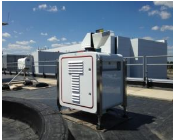
Figure 2: Picture of a New York State Mesonet upper air observation station located on the rooftop of the State University of New York in Albany, NY
