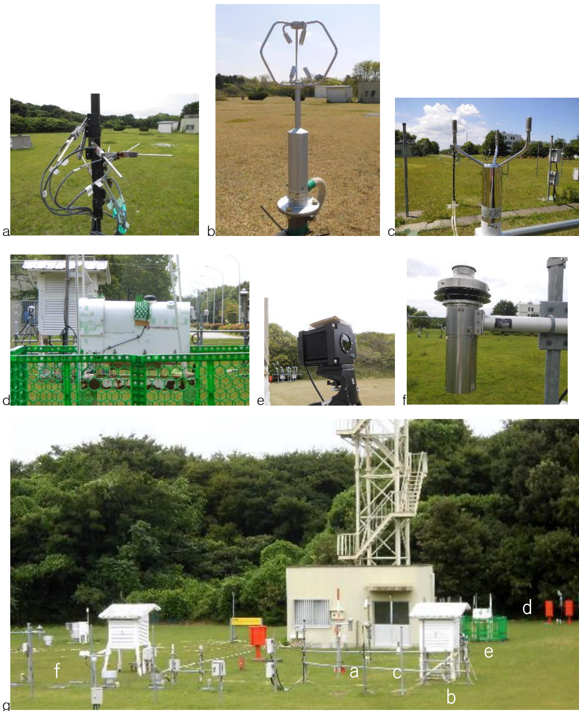
Figure 3. Instruments in the intercomparison study at the Meteorological Instrument Centre of Japan Meteorological Agency, Tsukuba, Japan. (a) Very thin thermocouples, (b) Ultrasonic SAT600, (c) Ultrasonic WMT701, (d) Radiometer MP-3000A, (e) Infrared camera VIM-384G2UL, (f) thermometer K5639AJ and hygrometer HMT333 within a JV-280 shield, and (g) a full view.
