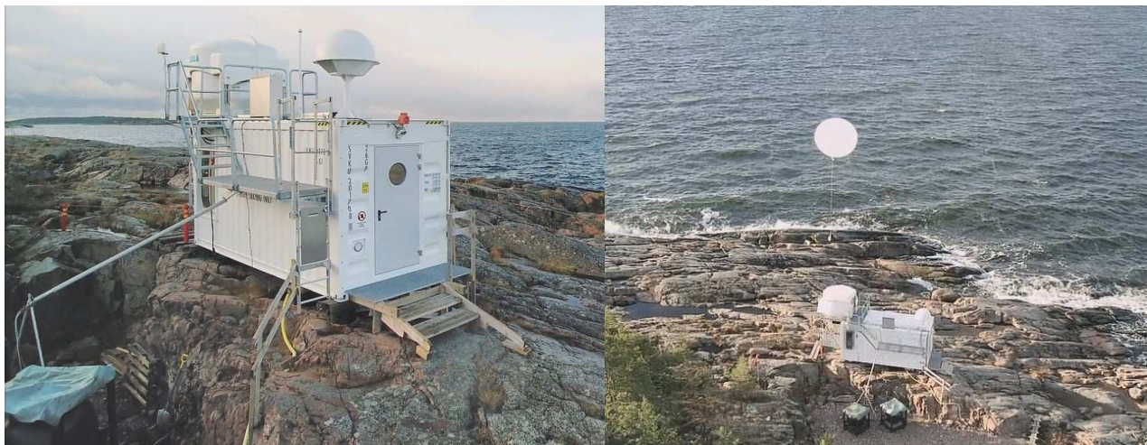
Figure 3. The newest design of an automatic sounding system, the new Vaisala AUTOSONDE AS41. Pictures are from a test site in the coast of the Gulf of Finland.
