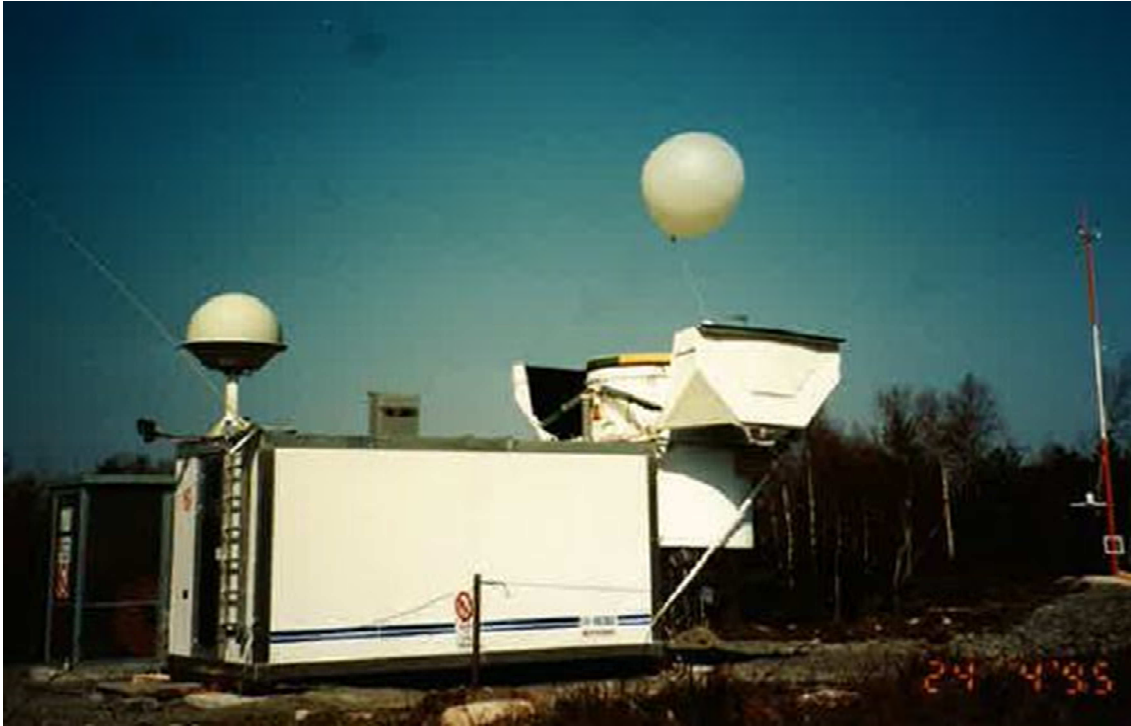
Figure 2. The first automatic sounding system in synoptic use by a WMO member, SMHI's Landvetter upper air station. The system was installed and commissioned in 1994. The photograph was taken in April 1995.
