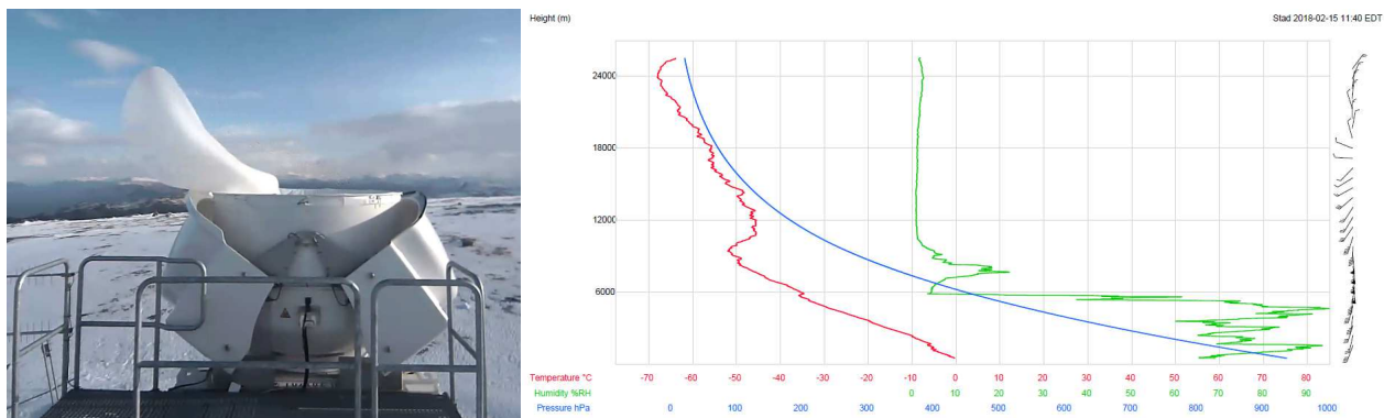
Figure 4. Left: Example of an RS41 launch with the new Vaisala AUTOSONDE AS41 in high wind condition in Vestkapp, Norway (wind speed 20.6 m/s at launch). Right: Sounding data profile from the same flight.
