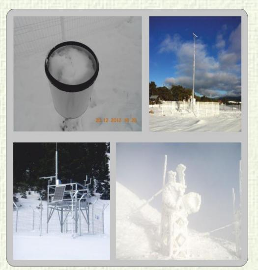
Freezing Prevention Equipment that installed as standart on measurement devices can't work in stations without grid electricity due to voltage mismatch.
