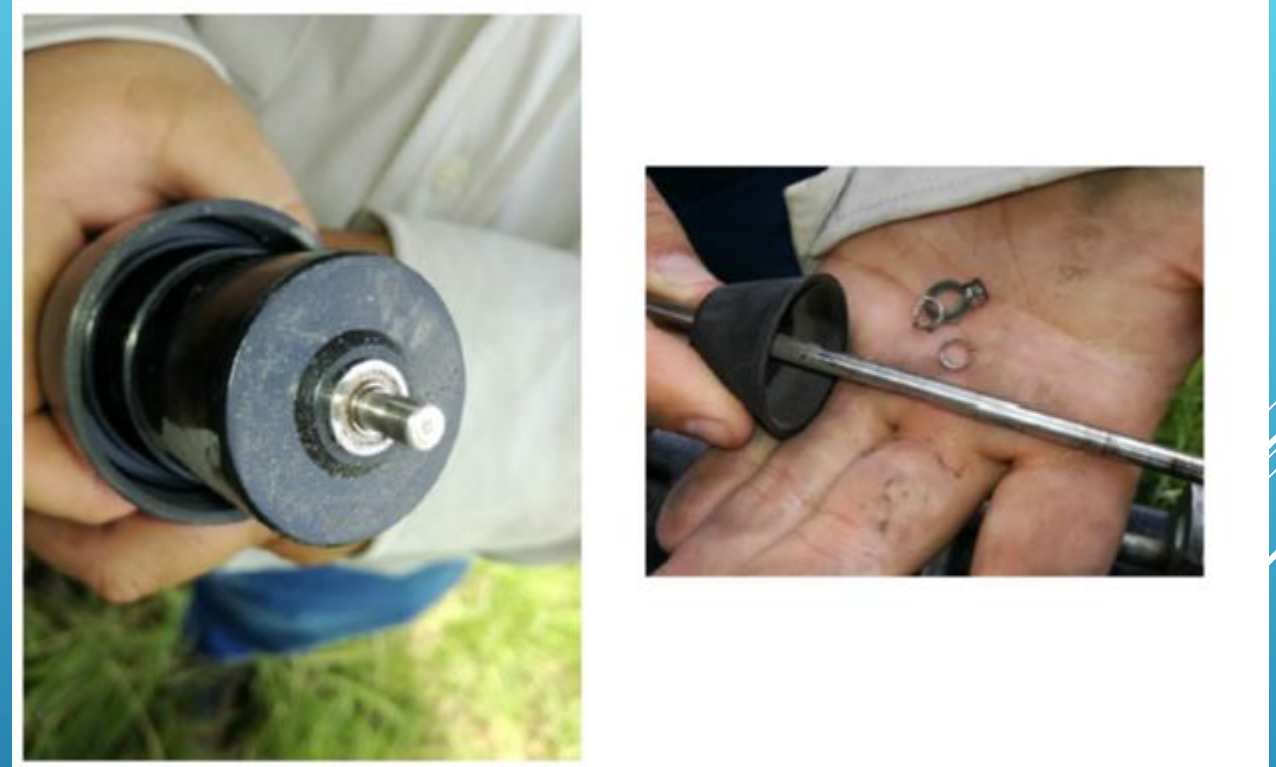
Rusted wind speed roles
