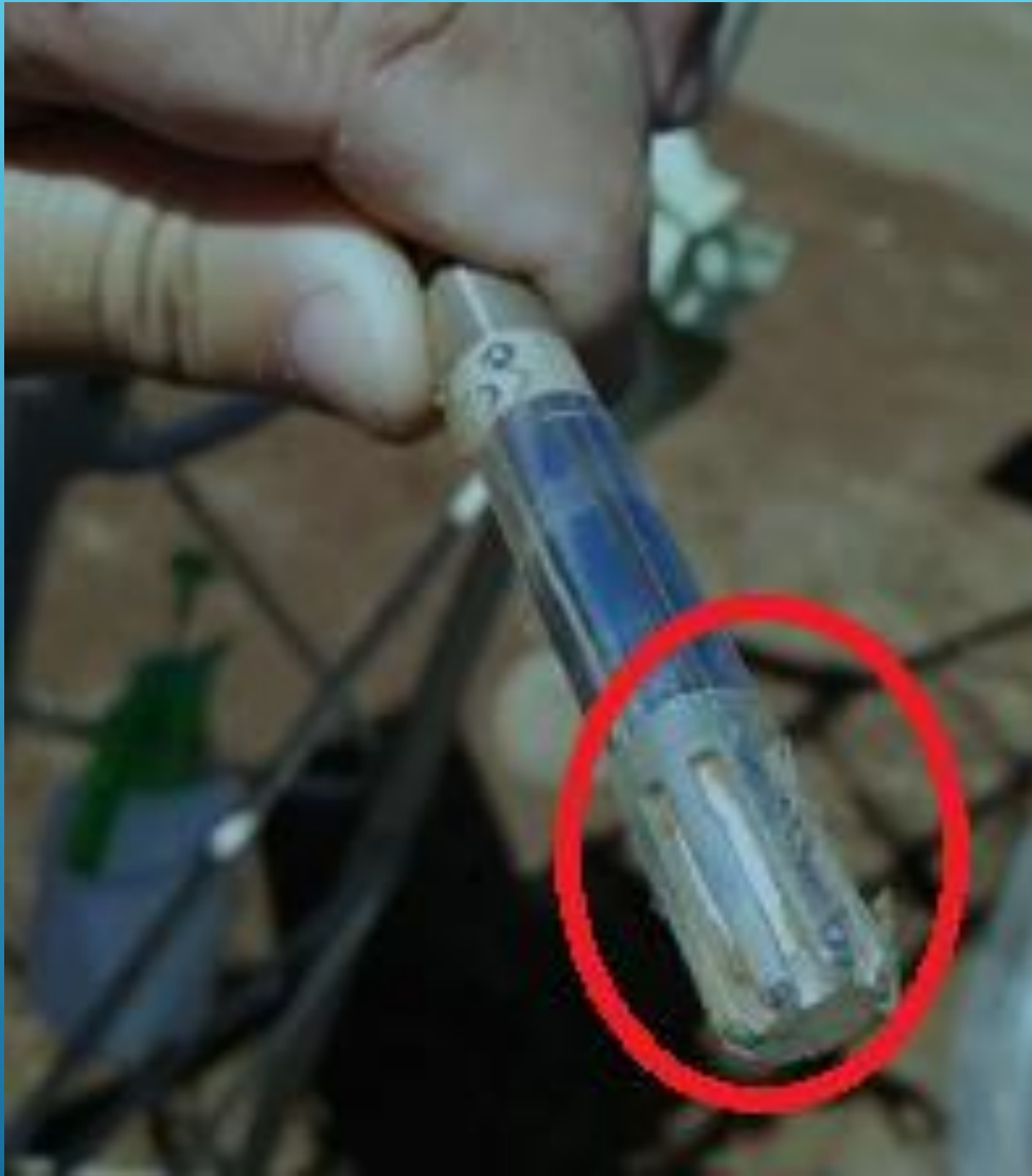
Mud panel on the temperature and humidity sensor.
