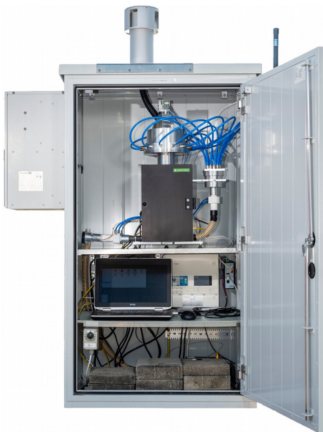
Figure 3: Swisens Poleno inside weatherproof housing
