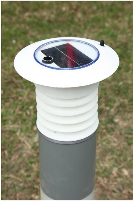
Figure 15 The solar-powered bollard type micro-climate measurement node at HKO Headquarters. Temperature, RH as well as UV Index are measured using this bollard. The small black disc at the top left hand side of the bollard is the UVI detector.
