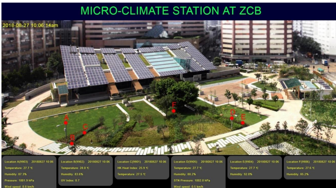
Figure 12 Locations of the measurement nodes and their respective measured weather elements at the micro-climate station at Zero Carbon Building in East Kowloon.
