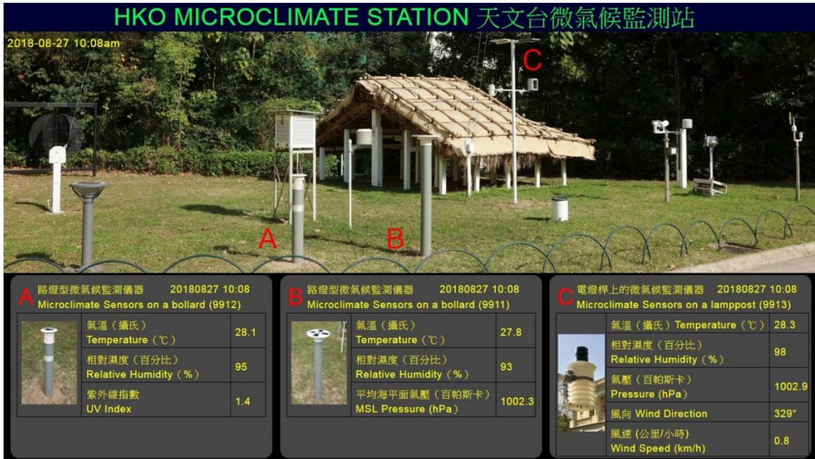
Figure 13 Locations of the measurement nodes and their respective measured weather elements at the micro-climate station at HKO Headquarters.
