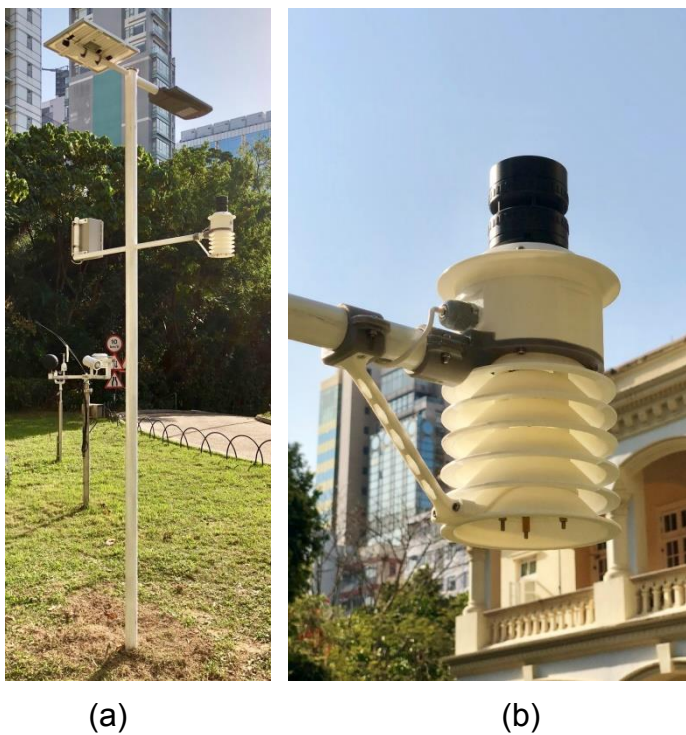
Figure 14 The prototype micro-climate measurement node mounted on a lamppost at HKO Headquarters (a). A close-up of the measurement node is shown in (b). The black cylinder-like object at the top is the ultrasonic anemometer. The white enclosure and radiation shield are made using 3-D printing technology.
