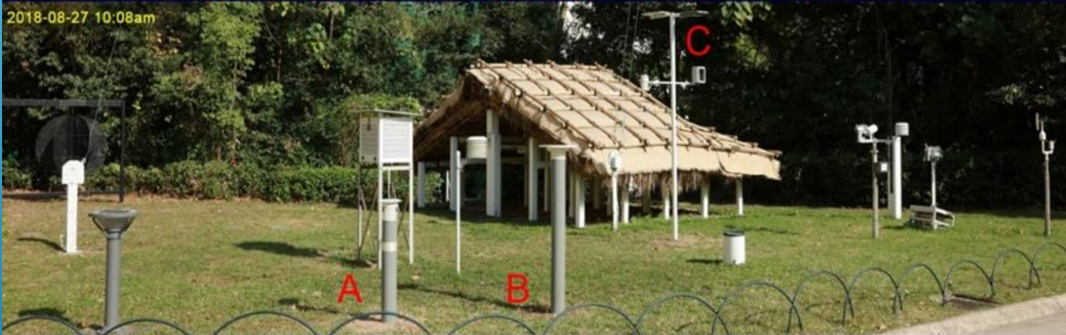
A 路燈型微氣候監測儀器 20180827 10:08 Microclimate Sensors on a bollard (9912)
