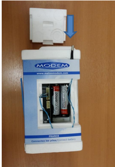
Fig.2. The optical radiosonde (photodiode is noted by blue arrow)
