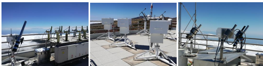
Figure 1: Spectroradiometers at the Izaña Observatory facility terrace (Tenerife, the Canary Islands, Spain).
