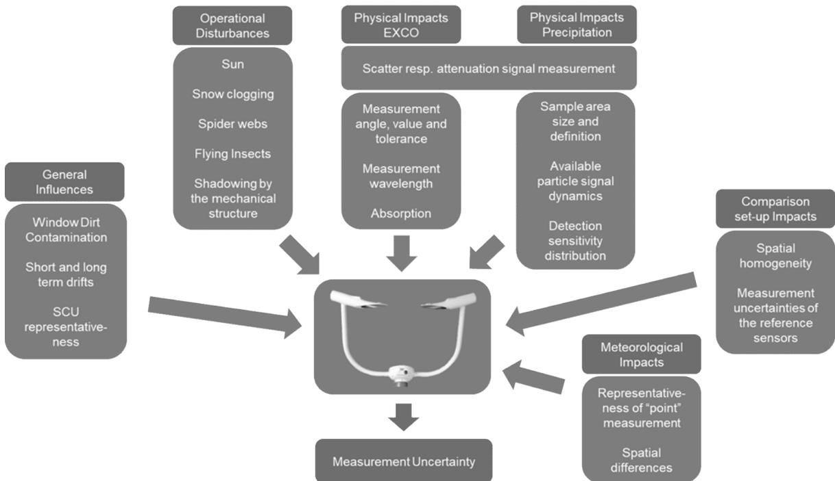
**Figure 4.** The measurement uncertainty sources of optical present weather and visibility sensors.
