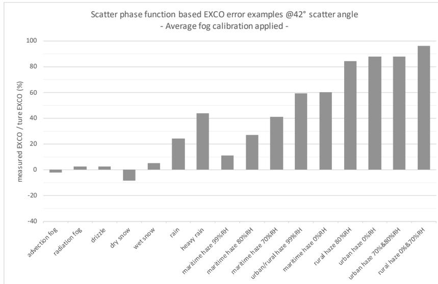
**Figure 16.** Scatter phase function based EXCO error examples for different phenomena.
