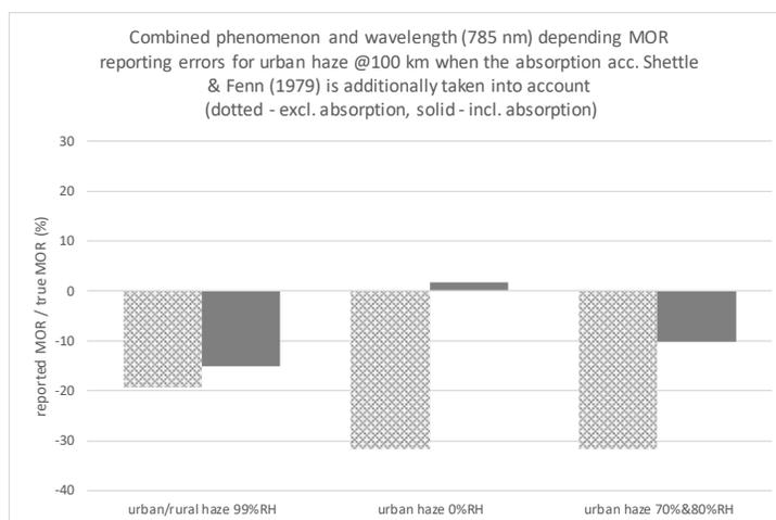
**Figure 23.** Combined phenomenon and wavelength depending impact on the reported MOR @100 km with and without absorption.
