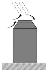
**Figure 8.** Under-catch due to upwind effects at a rain gauge.
