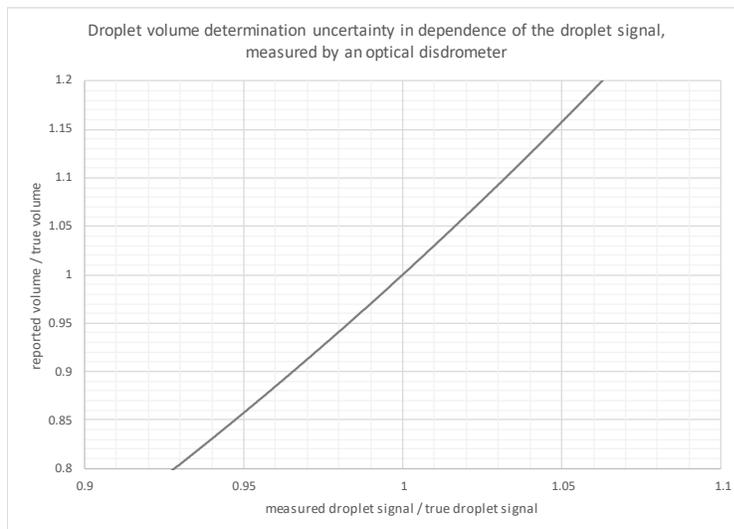
**Figure 12.** Droplet signal measurement error impact on the determined droplet volume for an optical disdrometer.
