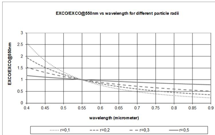
**Figure 18.** Measurement wavelength impact for different particle radii.
