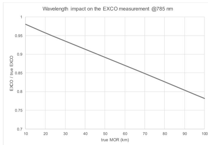
**Figure 19.** Wavelength impact on the EXCO, 785 nm example.
