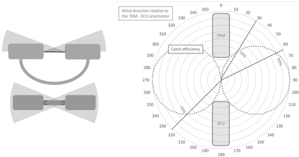
**Figure 7.** Sampling area shadowing of optical disdrometers.
