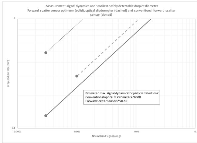
Figure 10. Impact of the effective light intensity on the small droplet detection capability.
