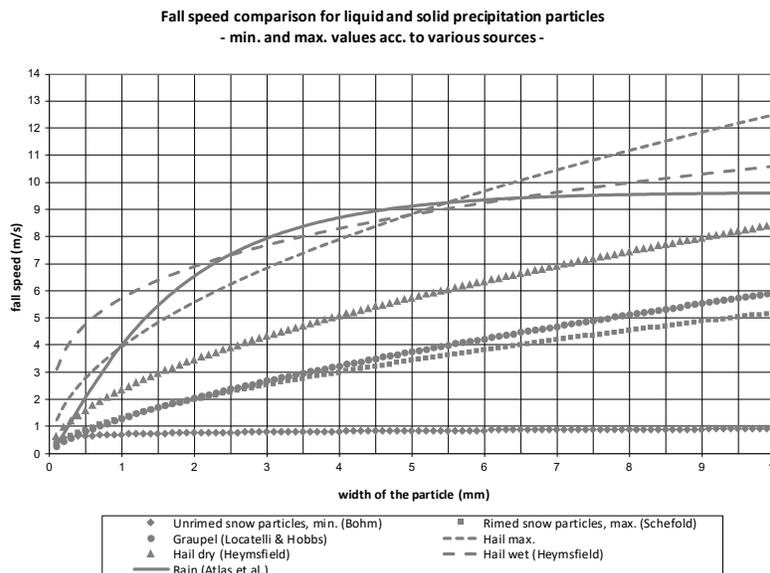
Figure 11. Fall speed examples for different precipitation particle types and sizes.
