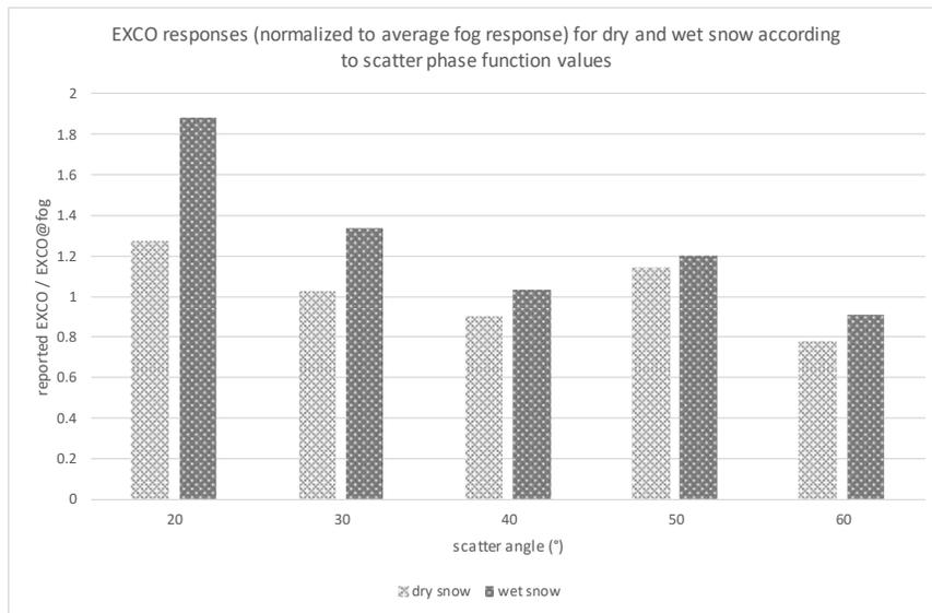
**Figure 15.** Scatter phase function based EXCO error examples for snow and different scatter angles.
