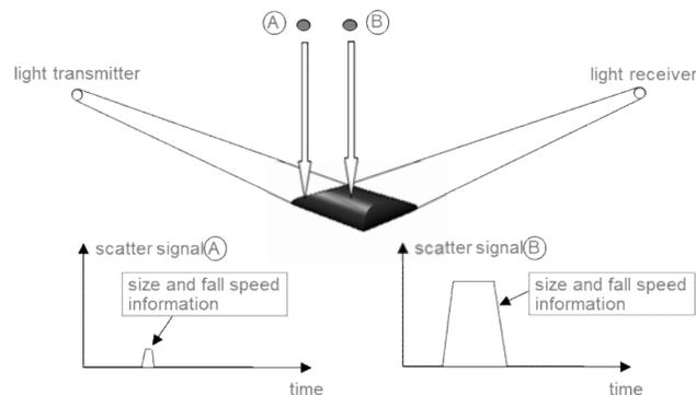
**Figure 3.** Droplet responses of an optical sensor in forward scatter geometry.
