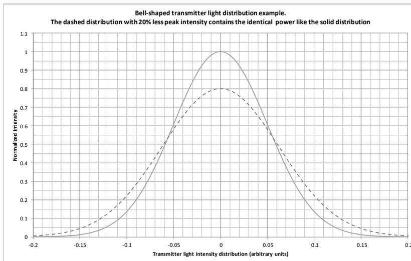
**Figure 13.** Bell-shaped transmitter light intensity distributions with different peak power, but identical total power.
