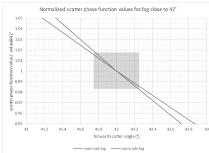
**Figure 17.** Fog scatter phase functions close to 42°.
