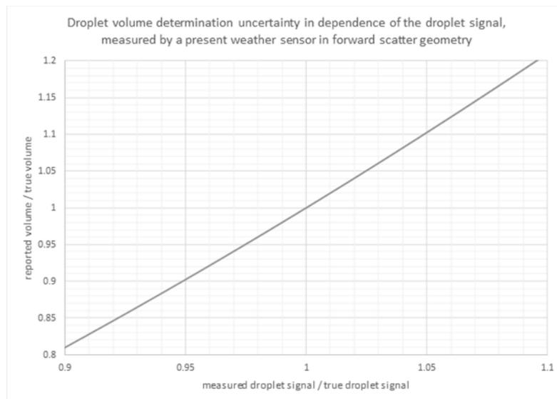
**Figure 5.** Droplet signal measurement error impact on the determined droplet volume for a forward scatter sensor.
