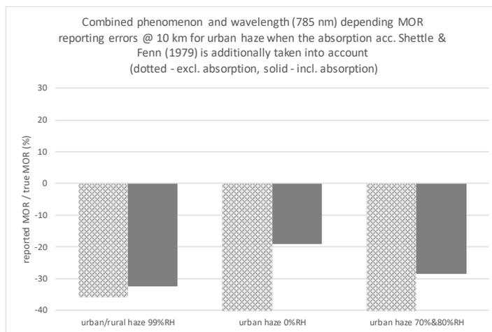
**Figure 22.** Combined phenomenon and wavelength depending impact on the reported MOR @10 km with and without absorption.
