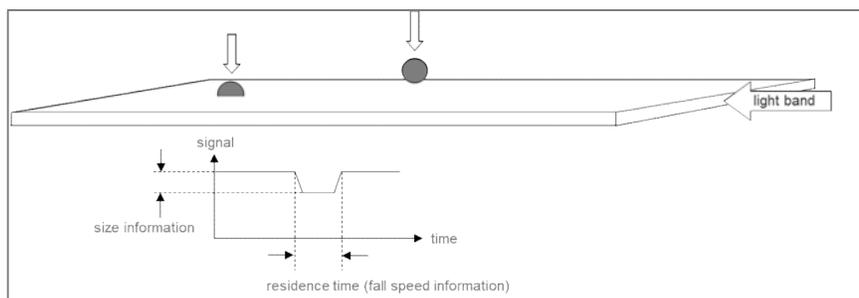
**Figure 2.** Optical disdrometer concept.
