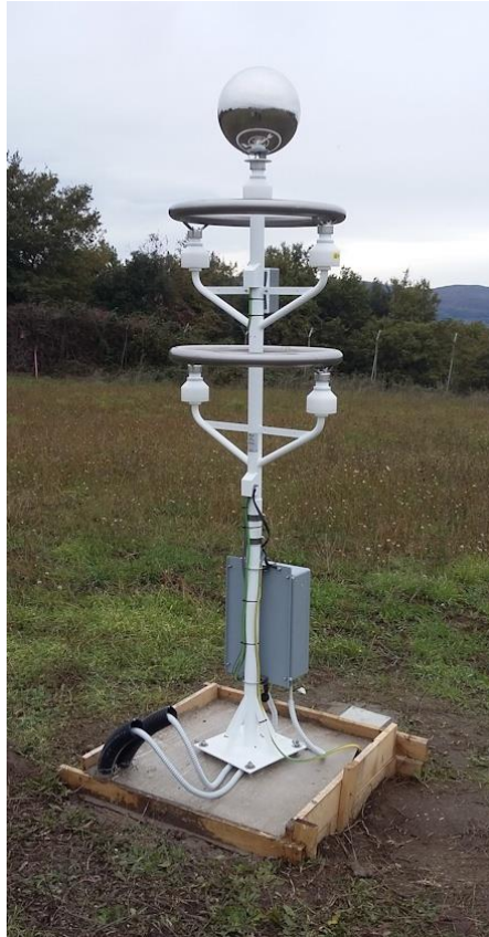
Figure 2: Biral BTM-300 thunderstorm detector installed at the WMO field intercomparison test bed in Vigna di Valle, Italy.
