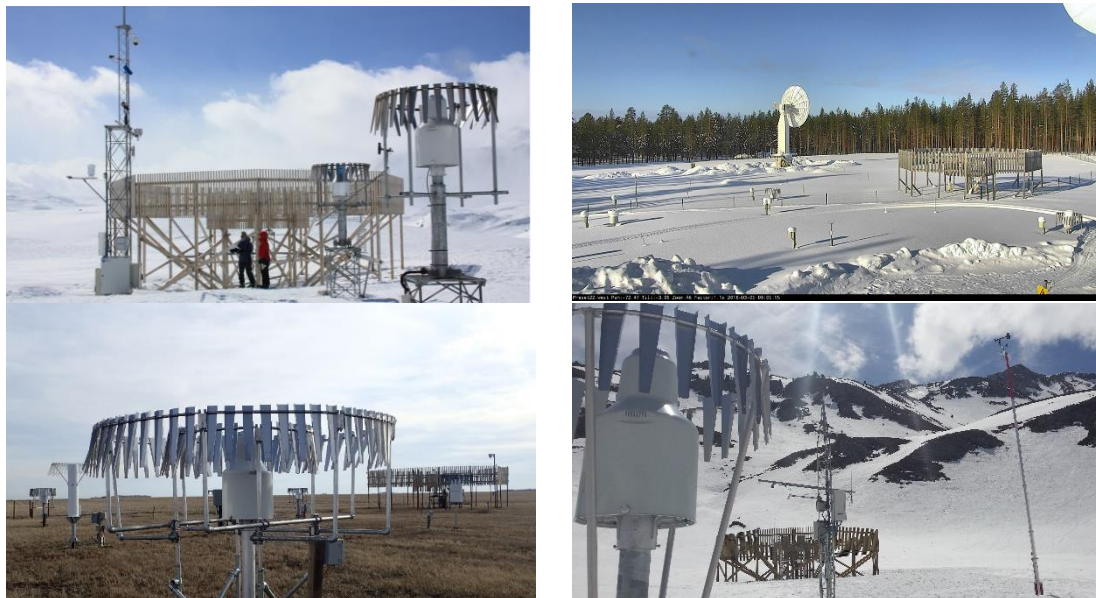
Figure 2. Site images. Top-left: Haukelisetter, Top-right: Sodankylä, Bottom-left: Bratt's Lake, Bottom-right: Formigal-Sarrios. The DFAR and weighing gauges in Single-Alter shields are observed.
