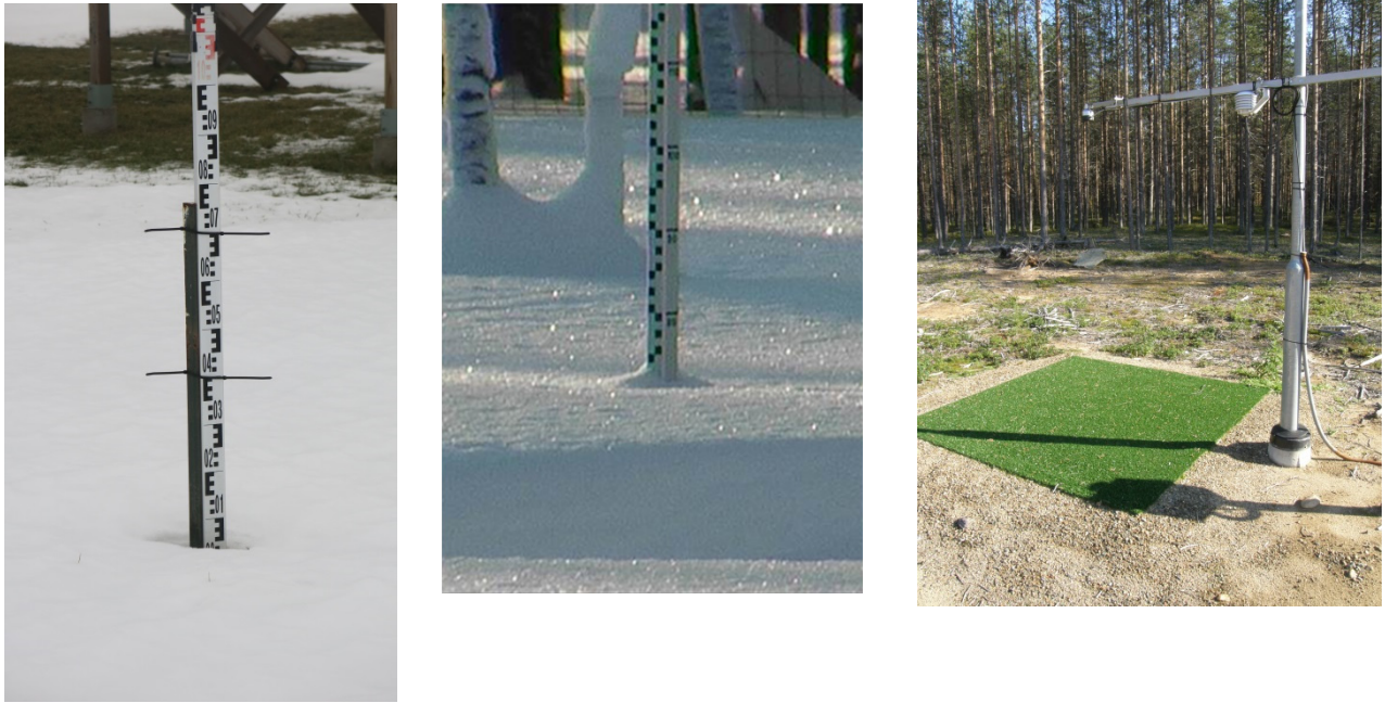
Figure 1: Left: visually observed snow stake; Middle: photographed snow stake; Right: sonic snow depth instrument over artificial target.
