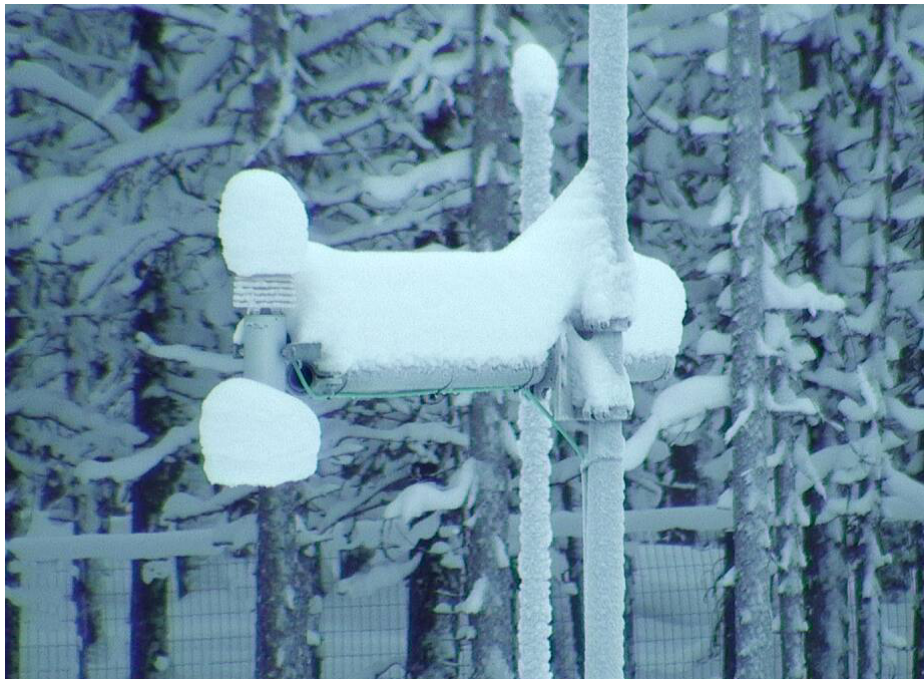
Figure 3: Unheated snow depth instrument and mounting infrastructure collecting snow in a low wind environment. (photo courtesy of FMI).
