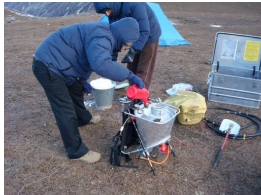
Figure 5: Left: A "hot-point drill" using steam produced in a pressure boiler, heated by propane. An insulated rubber hose, 10-15 m long, delivers steam to the drill stem. At a steam pressure of about 6 atmospheres, this drill penetrates 5-10 metres of ice per hour (Photo from Østrem and Brugman, 1991). Right: A lightweight, portable steam drill, suitable for use on high-altitude glaciers (Photo: Thorsteinn Thorsteinsson).
