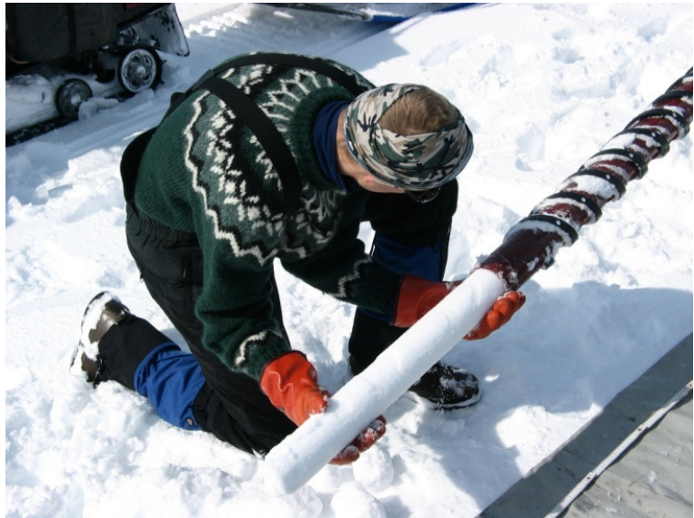
Figure 4: Left: A snow coring drill powered with a pipe threader in operation. Right: Removing a snow core from the core barrel (Photos: Thorsteinn Thorsteinsson).
