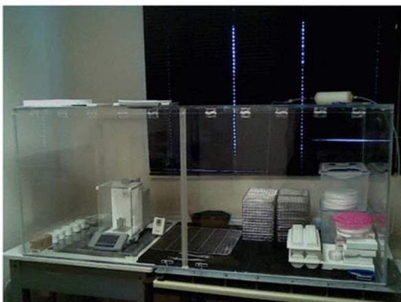
*Aerosol Filters laboratory: temperature and relative humidity controlled chamber*
