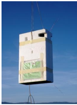
Figure 3 Meteolabor SRS-C34 radiosonde with original thermocouple temperature sensor fixed to thin wires that extend at a 45° angle upward (above right) and an additional thermocouple at a 45° angle downward (below right).
