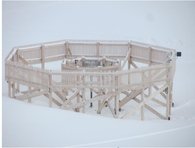
Figure 12 The reference measurement : the DFIR with an OTT Pluvio 2 weighing gauge on his center and a disdrometer. Other instruments for temperature, humidity, wind give ancillary data around the gauge measurement.
