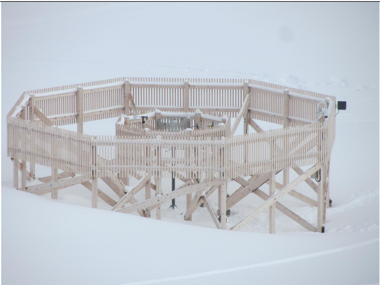
Figure 13 : The reference measurement : the DFIR with an OTT Pluvio 2 weighting gauge on his center and a disdrometer. Other instruments for temperature, humidity, wind give ancillary data around the gauge measurement.
