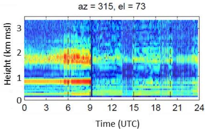
Figure 7: Ground clutter intensity as function of height. Strong echoes are observed at 1 and 2 km between 0 and 9h. At 9h an additional clutter fence panel has been installed which causes significant suppression of the clutter (see text).
