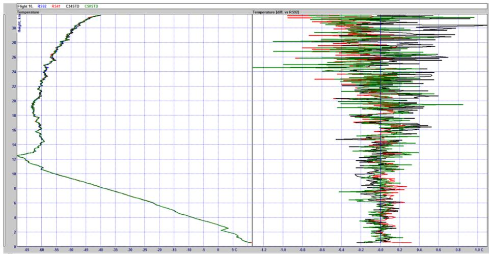
Figure 1. Comparison flight between various types of sondes including the new SRS-C50. Simultaneous temperature profiles (left panel) and temperature differences related to RS92 sonde (right panel).
