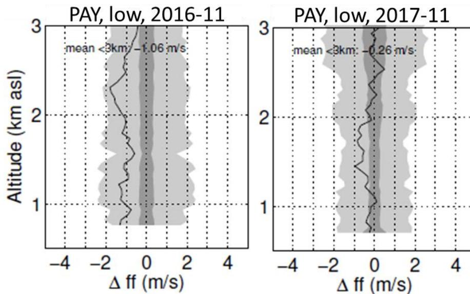
Figure 8: Bias (black solid line) and standard deviation (grey shaded area) of the differences between the radar windprofiler low mode and the operational radiosonde for November 2016 (left) and 2017 (right).
