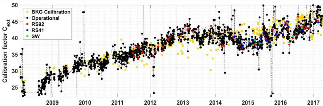
Figure 2: The time series of the water vapor calibration factor derived from the solar background and a reference calibration factor (yellow), derived from external calibrations using the operational radiosonde (black) and reference radiosondes (red, blue and green) respectively.
