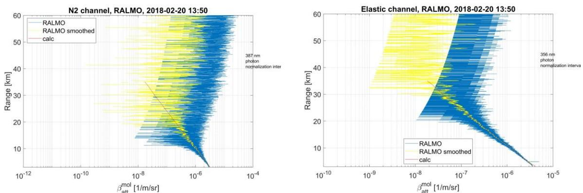
Figure 3: First measurements of the Raman lidar with the new laser source integrated over 30 min during daytime. Left panel: Nitrogen Raman channel, right panel: elastic channel.
