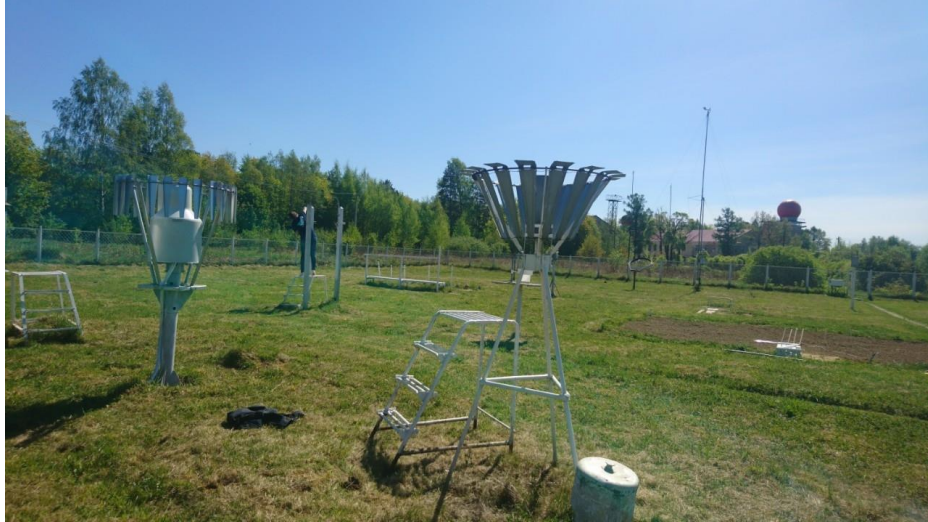
Precipitation gauge testing
