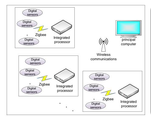
Integrated processing unit as an ISOS core integration components, mainly to complete the data processing, storage, transmission, control.
