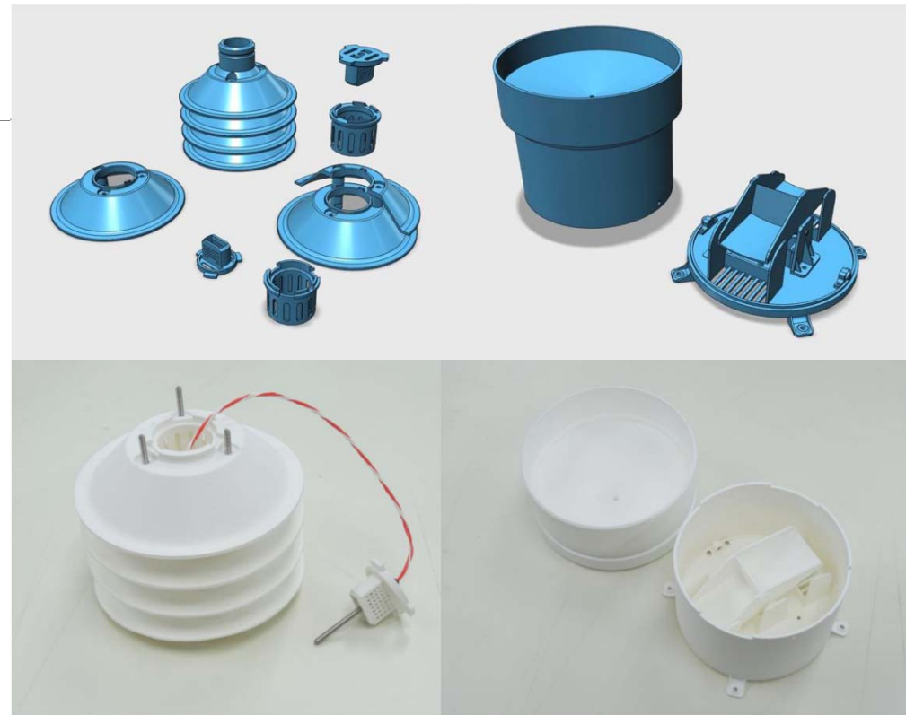
3D-printing radiation shield and tipping bucket raingauge (material: polylactic acid (PLA))
