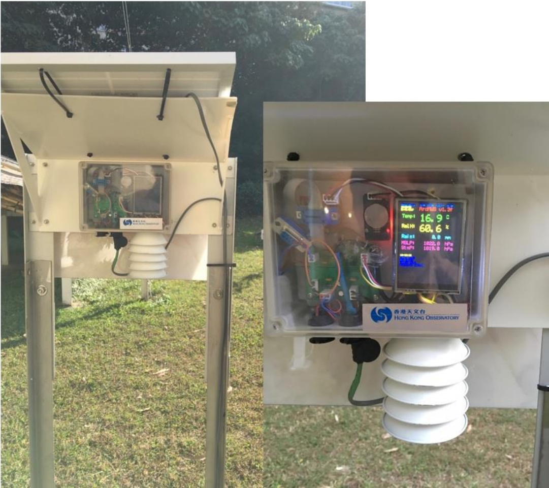
Figure 6 The prototype of a new generation Co-WIN 2.0 AWS installed in the field. Power is provided using batteries charged by a solar panel.
