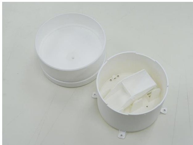
Figure 8 Accessories of a radiation shield and a small rain gauge designed for the AB-AWS using 3D printing (upper photos: computer images; lower photos: 3D printed products)
