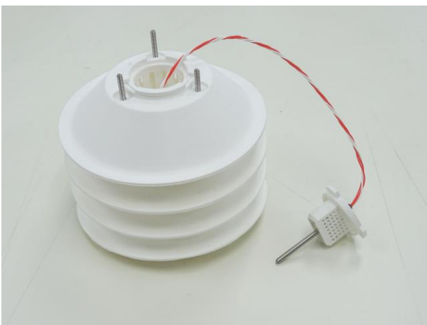
Figure 8 Accessories of a radiation shield and a small rain gauge designed for the AB-AWS using 3D printing (upper photos: computer images; lower photos: 3D printed products)
