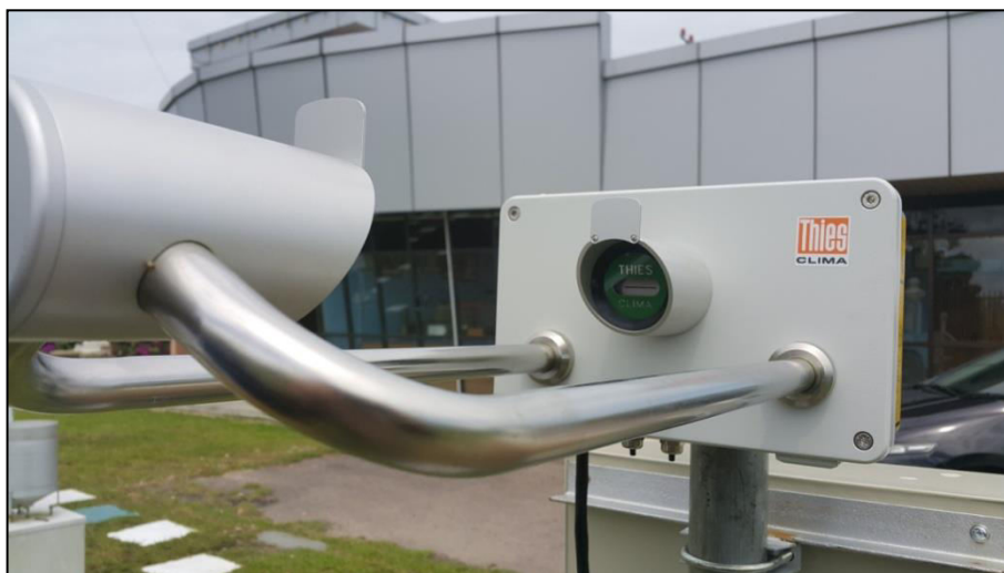
Figure 2.3. The Thies Laser Precipitation Monitor. The square box contains the laser diode and all electronic components, while the receiver is mounted in a small enclosure opposite to it.
