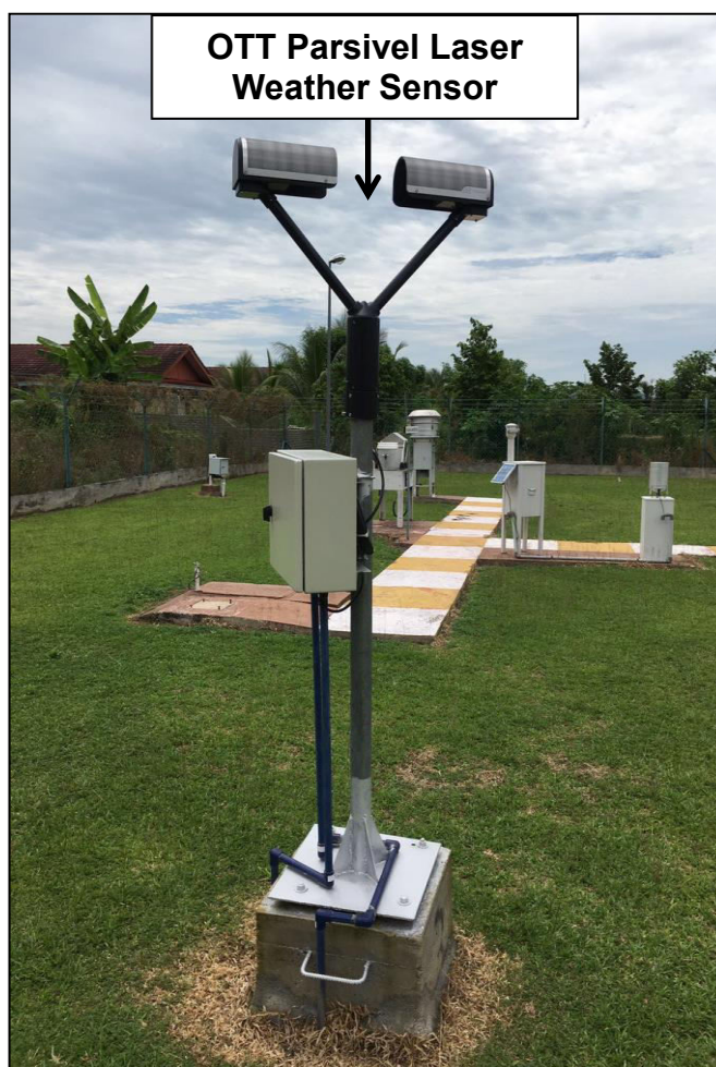
Figure B2. OTT Parsivel Laser Weather Sensor in Sitiawan Meteorological Station site.
