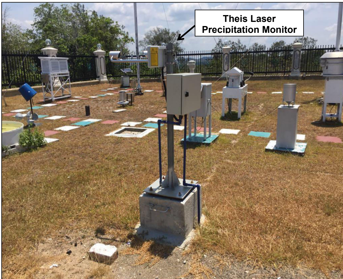
Figure B5. The Theis Laser Precipitation Monitor in Mersing Meteorological Station site.
