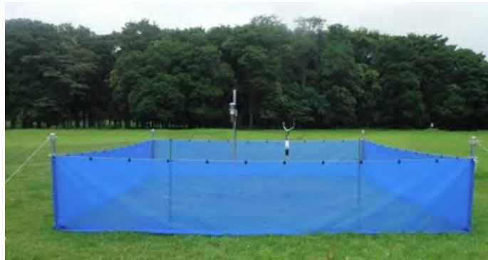
Figure 9 Observational field enclosed in a four-face net with a height of 1 m
