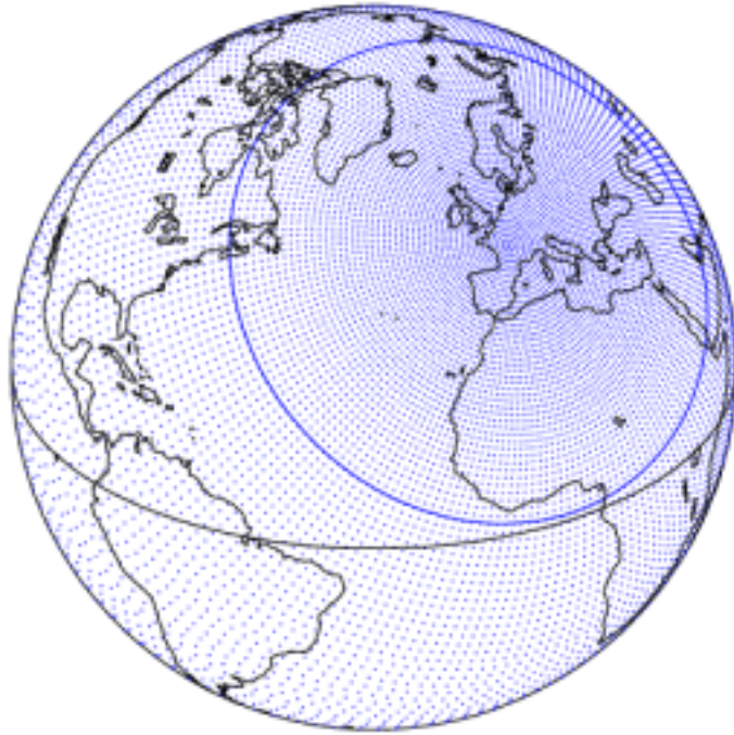
Figure 6. T358/c2.4 ARPEGE stretched grid as it is used in operations at Météo-France in 2004. The resolution varies from 23km over France to 133km at the antipode.
