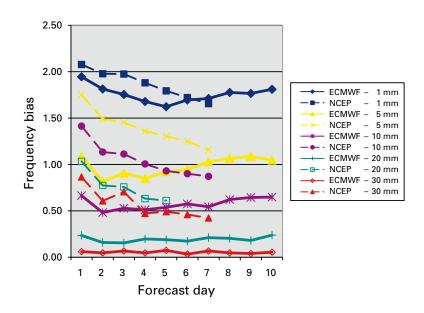
Figure 12. Frequency bias (B) for ECMWF (solid lines) and NCEP (dashed lines) forecasts of precipitation categories greater than 1-, 5-, 10-, 20- and 30-mm precipitation in 24 hours
