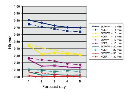
Figure 13. Hit rate (HR) for ECMWF (solid lines) and NCEP (dashed lines) forecasts of greater than 1, 5, 10, 20 and 30 mm in 24 hours for the 2010–2011 rainy season
