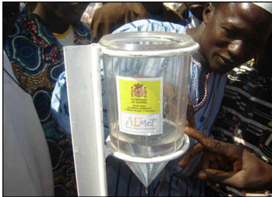
Figure 6.4 Incorrect positioning of the rain gauge (levelling).
