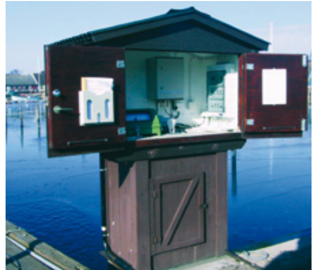
Figure I.4.12. Look-in type of instrument shelter over a stilling well
