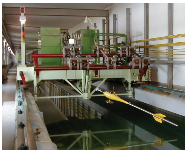
Figure I.5.21. Current meter rating tank located at the Swiss National Hydrological Survey calibration laboratory in Bern, Switzerland
