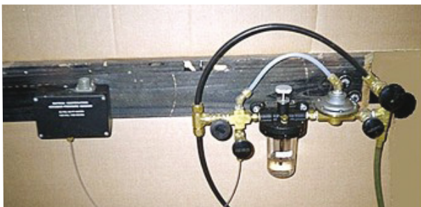
Figure I.4.27. Sutron Accububbler model 5600-0131-1 self-contained gas-purge system
