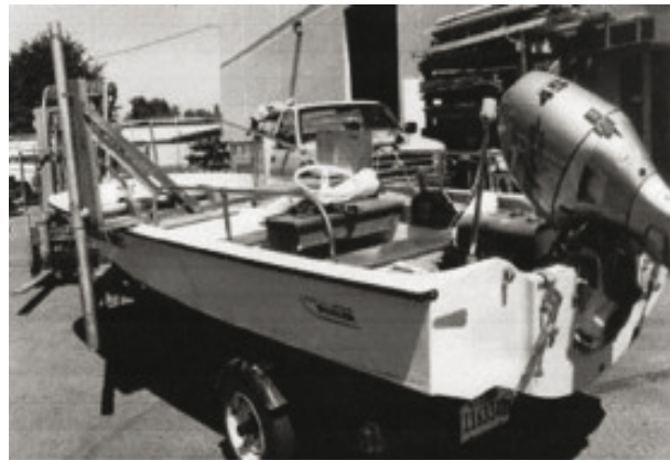
Figure I.6.12. Side-swing mount on a 4.5-metre Boston Whaler for an ADCP
