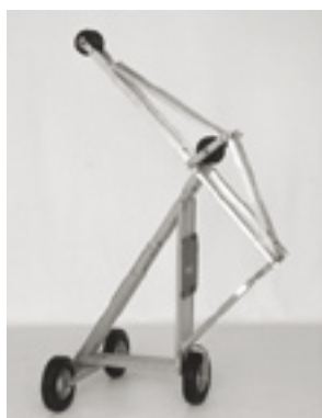
Figure I.5.54. Type A crane mounted on a 3-wheel base
