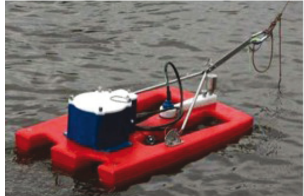
Figure I.6.9. An RD Instruments Streampro ADCP mounted on a small tethered boat
