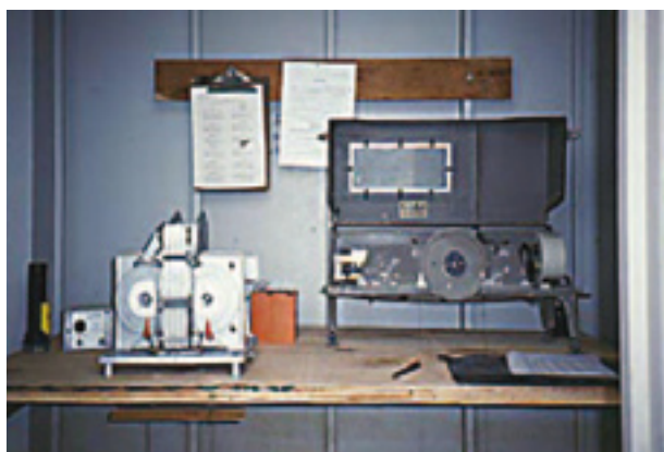
Figure I.4.34. Stevens analog digital recorder (left) and Stevens A-35 strip-chart recorder (right)
