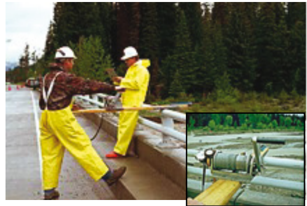
Figure I.5.53. Measuring from a bridge with a bridge board
