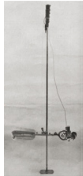
Figure I.5.27. Round wading rod with meter attached
