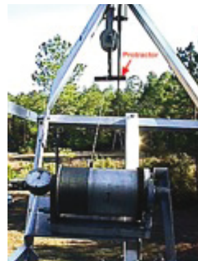
Figure I.5.56. Protractor used for measuring vertical angles
