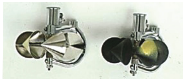
Figure I.5.6. Price AA meter with winter-style yoke and polymer rotor
