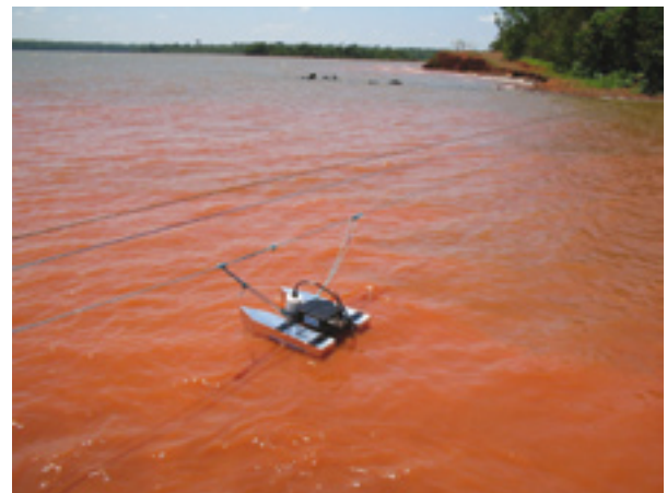
Figure I.6.14. A temporary bank-operated cableway for making ADCP measurements with a tethered ADCP boat
