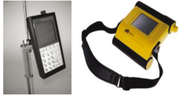
Figure I.5.61. Electronic field notebooks, Aquacalc Pro (left) and Ott Vota-2 (right)
