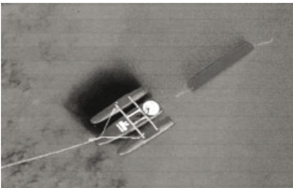
Figure I.6.15. Tethered ADCP boat with a sea anchor attached
