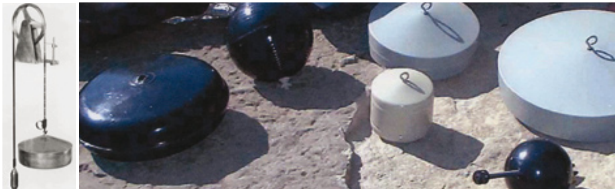
Figure I.4.19. Float-tape gauge and various float types
