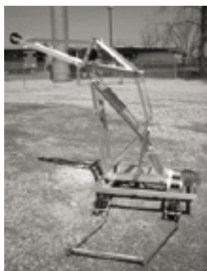
Figure I.5.55. Type E crane mounted on a 4-wheel base
