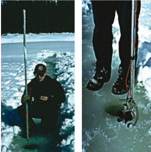
Figure I.5.68. Ice rod being used to support current meter for a discharge measurement (left); Price AA current meter with polymer rotor used for ice measurements (right).
