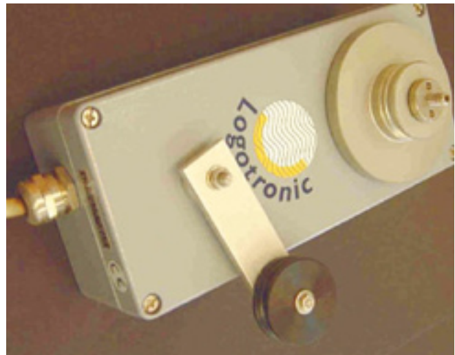
Figure I.4.22. Design Analysis Associates WaterLOG model H-510 shaft encoder (left) and the Logotronic Gealog shaft encoder (right)
