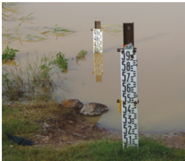
Figure I.4.13. Standard metric, outside, vertical staff gauge, attached to 2 x 6 wood backing
