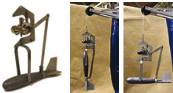
Figure I.5.59. Ice measurement supports, and tilting harness for 30-pound C-type weight
