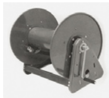
Figure I.5.42. Horizontal-axis boat tag line reel without a brake
