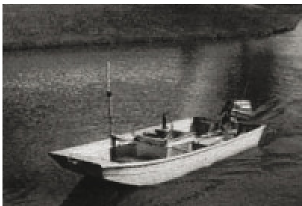
Figure I.6.16. Radio controlled ADCP platform, 3.6 metres boat
