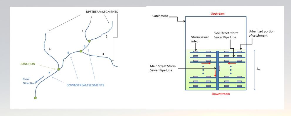
$$\partial y/\partial t + \partial (vy)/\partial x = 2q_{L}/B - f$$
