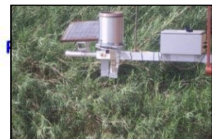
Automatic Radar River Level Stations • Flood monitoring equipment • Early detection of dangerous water levels
