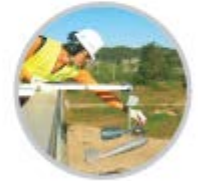
Measurement by floats and bridge board
