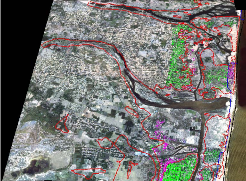
Building polygons are in hazard area (pink) and non-hazard area (green) are overlaid
