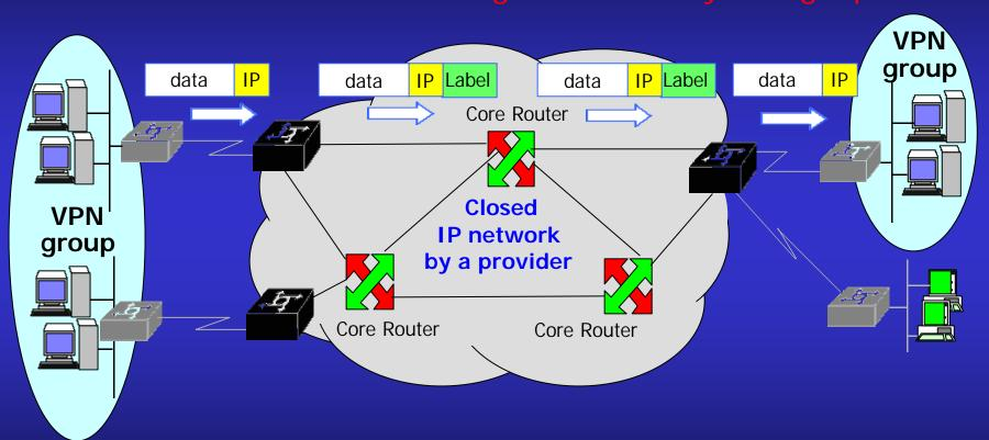
IP-VPN with MPLS provides any to any connectivity within a VPN group, a guaranteed quality of service, reliability, scalability of capacity and full security.
