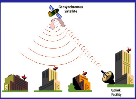
One Way VSAT system is used for broadcast/multicast.
