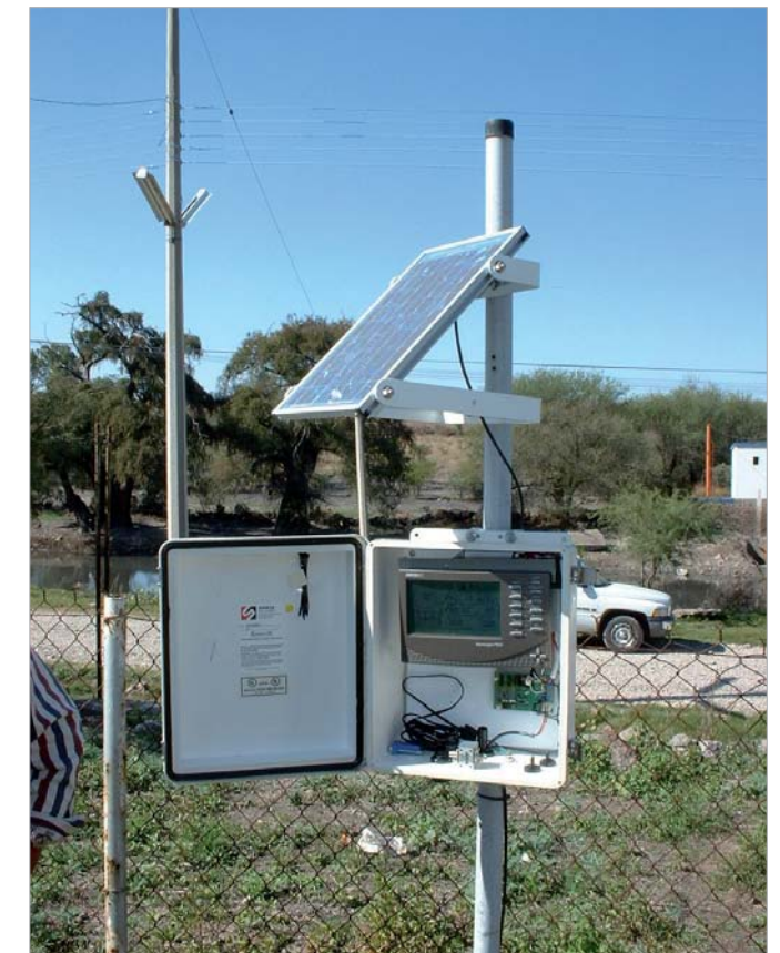
The meteorological information is crucial for an adequate management of water resources. Above, Hurricane approaching Mexico. Below, Automatic Weather Station of the Mexican network (photos PROMMA).
