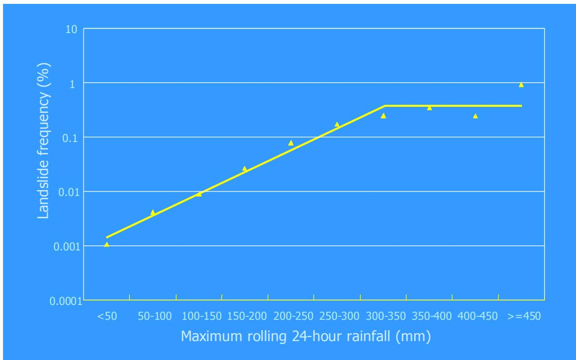
Fig. 6 Overall correlation between landslide frequency and maximum rolling 24-hour rainfall for soil cut slopes in Hong Kong.
