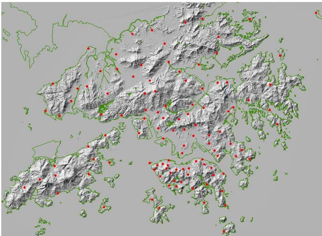
Fig. 8 Locations of automatic raingauges managed by GEO and HKO.
