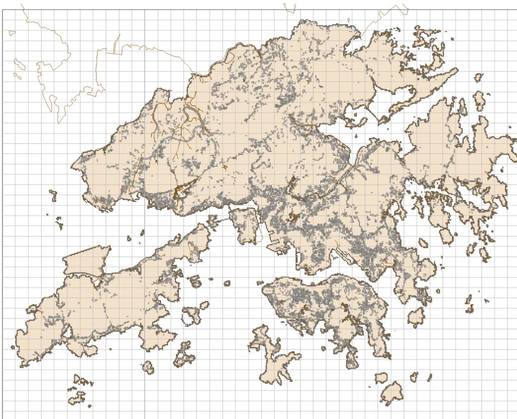
Fig. 4 Spatial distribution of man-made slopes (grayed areas) in Hong Kong. The grid lines indicate the discretization of the territory into 1,600 cells.
