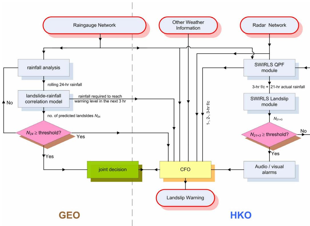
Fig. 7 Major information flow in landslide warning operation.
