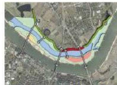
Figure 2: The 'Room for the River' plan at Nijmegen. The green line indicates the current line of the protective dike. The red line shows the position of the proposed relocated portion of dike. In the bottom image, the new river channel is shown in blue and the new island in yellow-green. The white arrows represent the bridge connections planned for the island. Source: Nijssen and Schouten, 2012<sup>13</sup>.
