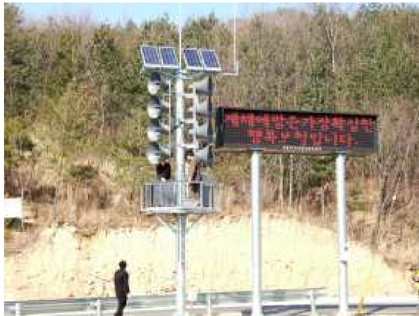
<Figure 2. Observation Station for the Rainfall Warning System>
