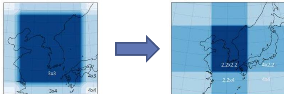
Figure 12. LENS domain with 3x3 km (left) and new domain with 2.2x2.2 km spatial resolution
