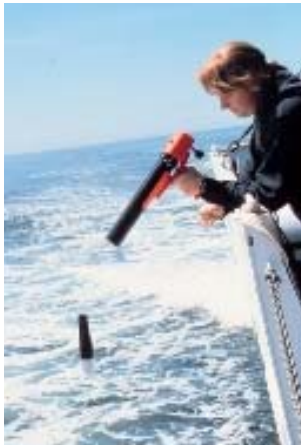
Expendable bathythermographs sample the structure of the upper layers of the ocean.
