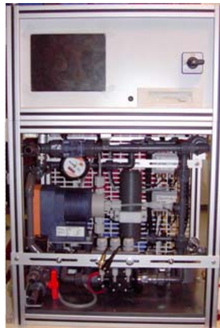
Pressure resistant FerryBox II (closed system)
