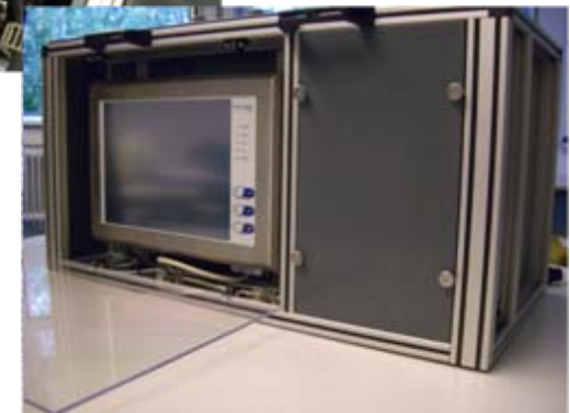
Transportable „Pocket FerryBox“ For field campaigns aboard small boats
