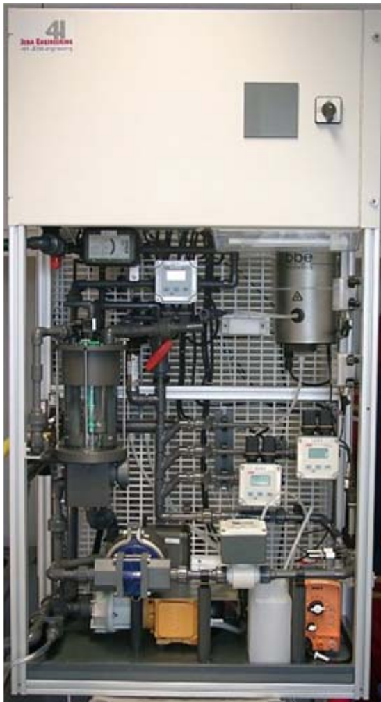
Standard FerryBox incl. debubbler
