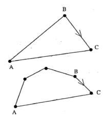
Position "FROM" A: "DR" position B: C: Position "TO" AB: True course steered. corrected for leeway and distance run Course and distance made AC: good Current set and drift BC:
