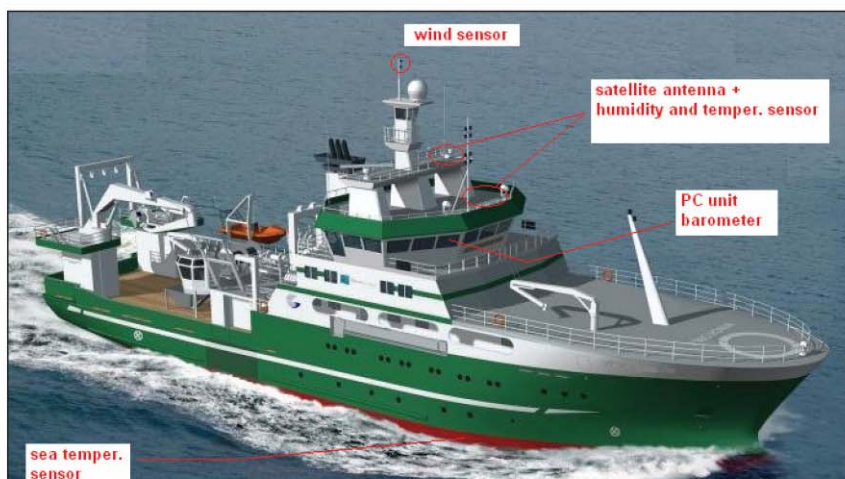
▲ Figure 1: Batos II instrument layout schematic
