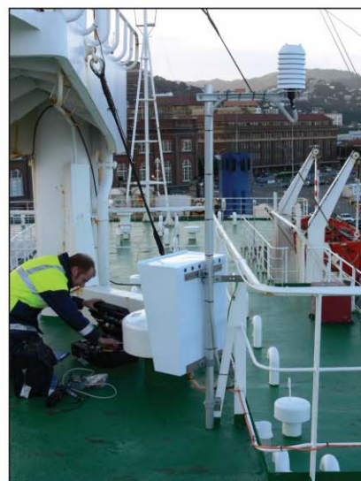
▲ Figure 3: mStar-Ship AWS console and temperature screen on board Spirit of Competition
