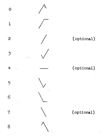
N o t e : The slanting part of the symbols should make an angle of about  $30^{\circ}$  with the vertical.
